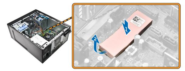
5 Slide the PCle SSD card into the slot and tighten the screw to secure the card to the system board [1,2].
