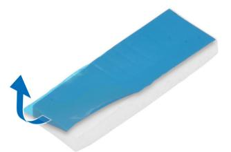
4 Place the thermal pad in the slot on the system board and peel the pink adhesive tape [1,2].
