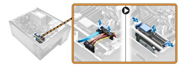
5 Flex the hard drive bracket and remove the hard drive from the hard drive bracket.
