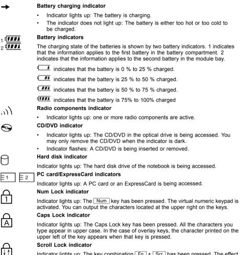
Indicator lights up: The key combination Fn + Scr has been pressed. The effect this key has varies from programme to programme.
