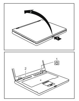
Press the release button (1), and unfold the LCD screen upwards (2).
