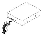
Figure 20. Connecting a SATA optical drive
