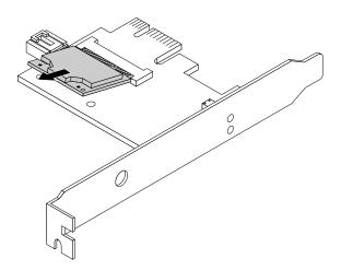
Figure 39. Removing the WiFi card module
