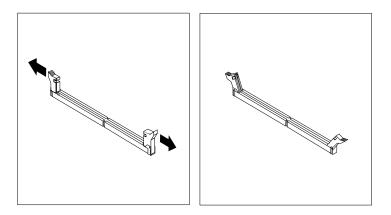
Figure 16. Opening the retaining clips
