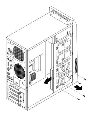
Figure 29. Removing the hard disk drive
