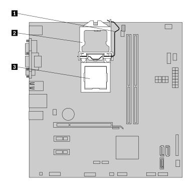
Figure 25. Accessing the microprocessor
