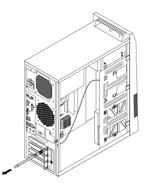
Figure 44. Removing the rear WiFi antenna
