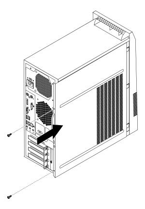
Figure 50. Reinstalling the computer cover
