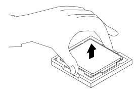
Figure 26. Removing the microprocessor
