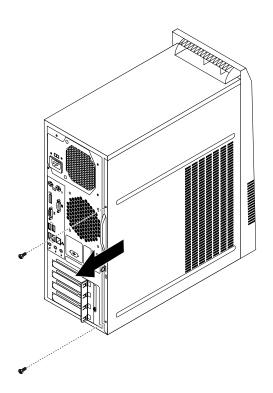
Figure 9. Removing the computer cover
