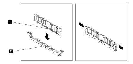
Figure 17. Installing a memory module
