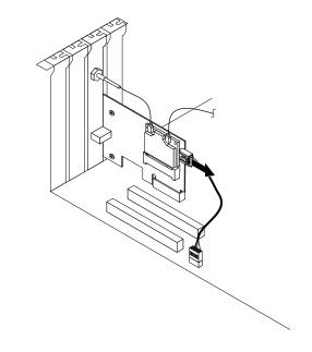
Figure 35. Disconnecting the Bluetooth cable
