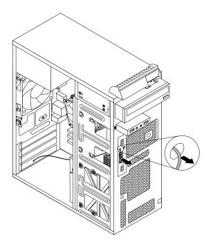
Figure 47. Removing the front WiFi antenna
