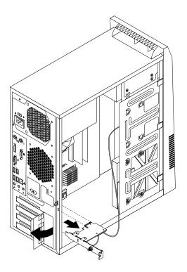
Figure 36. Removing the WiFi adapter card
