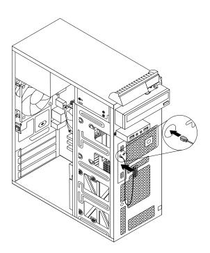
Figure 46. Installing the front WiFi antenna
