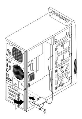
Figure 42. Installing the WiFi adapter card
