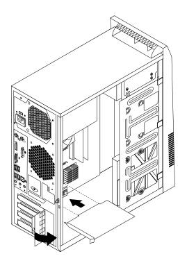
Figure 14. Installing a PCI Express card
