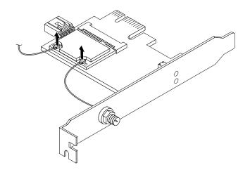
Figure 37. Removing the WiFi antenna cables
