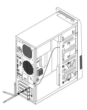
Figure 43. Installing the rear WiFi antenna
