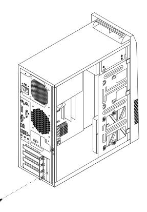
Figure 12. Removing the screw that secures the PCI Express card latch
