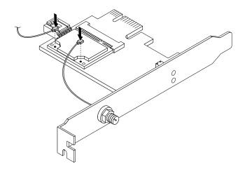
Figure 41. Installing the WiFi antenna cables
