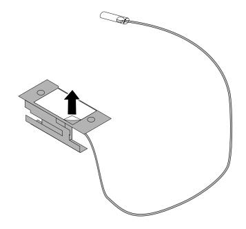
Figure 45. Peeling off the paper that protects the stickers
