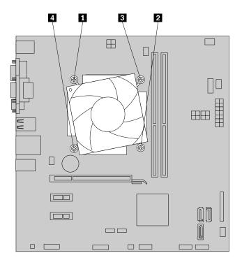
Figure 23. Removing the heat sink and fan assembly
