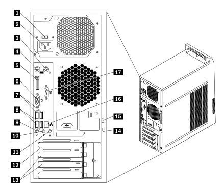
Figure 2. Rear connector locations
