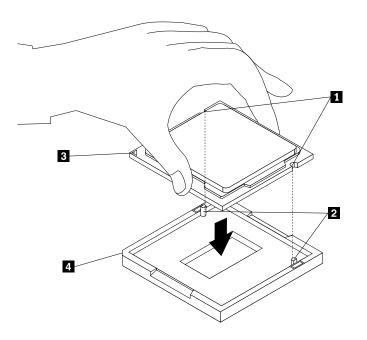
Figure 27. Installing the microprocessor
