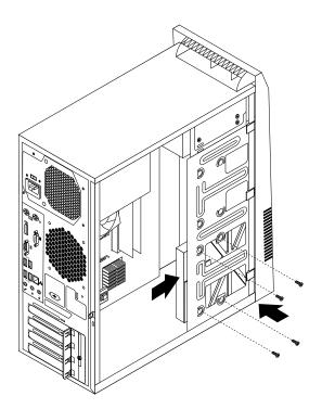
Figure 30. Installing the hard disk drive
