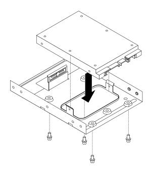
Figure 28. Installing the solid-state drive into the storage converter
