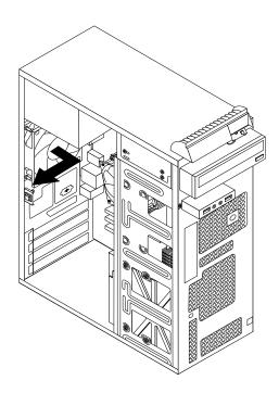
Figure 32. Removing the rear fan assembly
