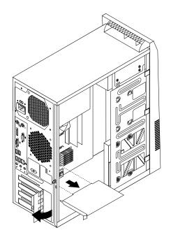
Figure 13. Removing the PCI Express card
