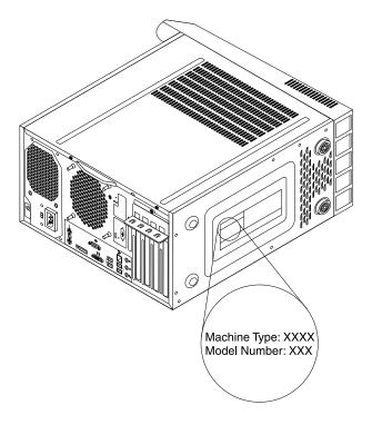
Figure 6. Machine type and model label
