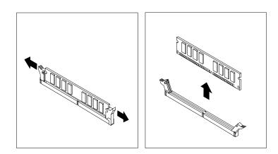
Figure 15. Removing a memory module
