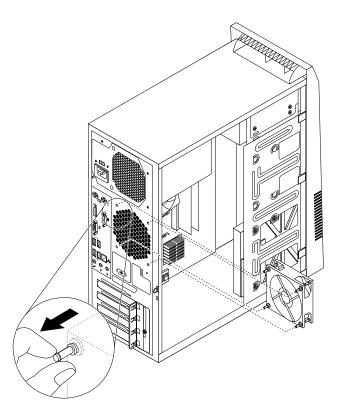
Figure 33. Installing the rear fan assembly
