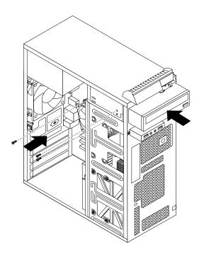
Figure 19. Installing the optical drive
