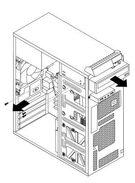
Figure 18. Removing the optical drive
