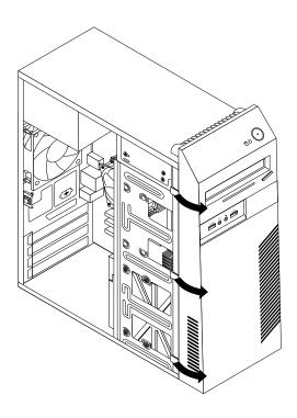
Figure 10. Removing the front bezel
