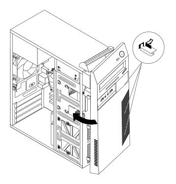
Figure 11. Reinstalling the front bezel
