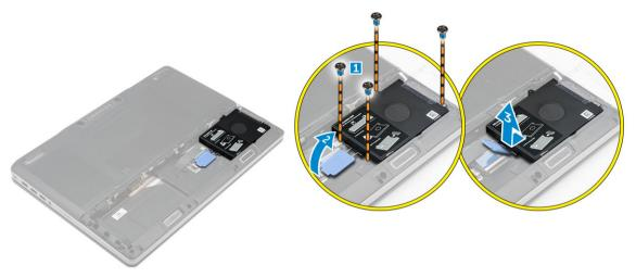
4 Remove the screws that secure the hard drive. Lift the hard drive from the bracket.
