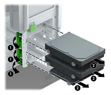
5. Remove the four mounting screws (two on each side) from the old drive. You will need these screws to install a new drive.
