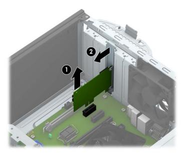
**c.** If you are removing a PCI Express x16 card, pull the retention arm on the back of the expansion socket away from the card and carefully rock the card back and forth until the connectors pull free from the socket. Lift the card straight up then away from the inside of the chassis to remove it. Be sure not to scrape the card against other components.
