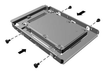
Install four 6-32 silver and blue isolation mounting screws in the adapter bracket (two on each side of the bracket).
