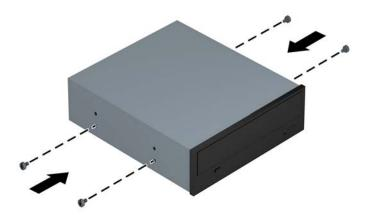
Slide the drive into the drive bay, making sure to align the mounting screws with the mounting slots, until the drive snaps into place.
