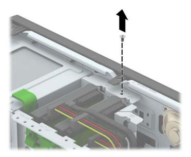
4. Install the security screw through the middle front bezel release tab to secure the front bezel in place.
