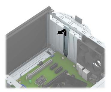
**b.** If you are removing a standard PCI card or PCI Express x1 card, hold the card at each end and carefully rock it back and forth until the connectors pull free from the socket. Lift the card straight up (1) then away from the inside of the chassis (2) to remove it. Be sure not to scrape the card against other components.
