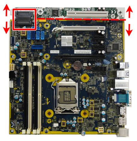
When reinstalling the system board, first insert the I/O panel back into the slots in the rear of the chassis, and then align the board with the chassis screw holes.
