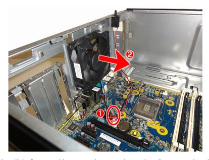
To install the fan assembly, reverse the removal procedure. Be sure to orient the air flow out of the unit.
