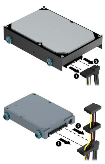
4. Remove the drive by pulling the release tab away from the drive (1) and sliding the drive out of the bay (2).
