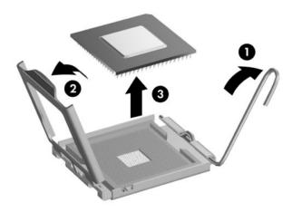
Reverse the removal procedure to install a new processor.
