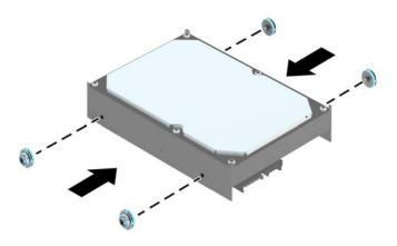
• If you are installing a 2.5-inch hard drive, install four black and blue M3 isolation mounting screws (two on each side of the drive).
