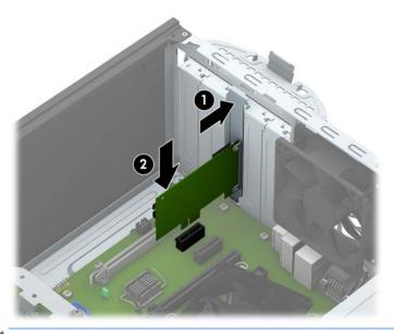
NOTE: When installing an expansion card, press firmly on the card so that the whole connector seats properly in the expansion card socket.
