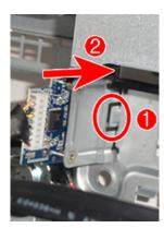
To install the card reader, reverse the removal procedures.
