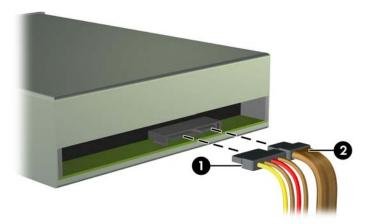
CAUTION: When removing the cables, pull the tab or connector instead of the cable itself to avoid damaging the cable.
