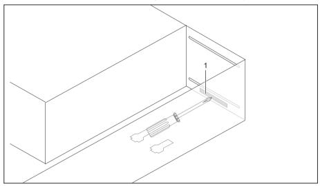
Break out the pre-stamped metal cover (1) with a screwdriver.
