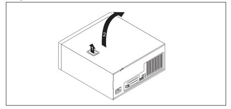
▶ Pull the locking device (1) and swivel the side part in the direction of the arrow (2).
