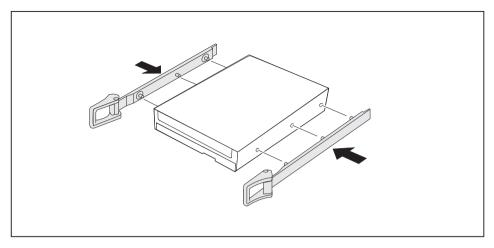
Secure the EasyChange rails on the side of the hard disk by inserting the upper pins of the EasyChange rail in the corresponding holes on the hard disk.
