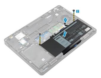
4 Unroute the cable from the routing channel [1] and remove the cable from the battery [2].
