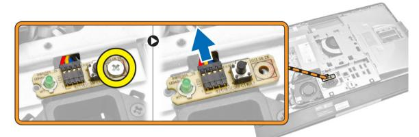
4. Remove the screws that secure the power connector to the I/O board shield.
