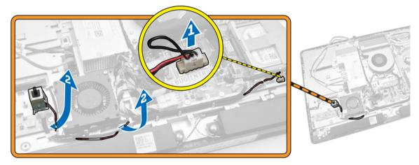
4. Remove the screws that secure the intrusion switch to the chassis. Lift the intrusion switch and remove it from the computer.
