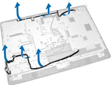
5. Remove the screw that secure WEB GND cable. Remove the tape from both sides of the display panel.
