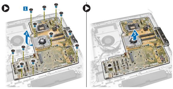
5. Lift and remove the system board from the chassis.
