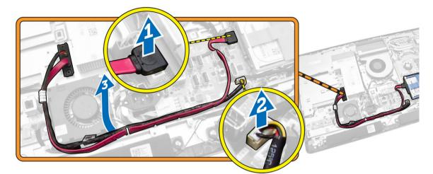
5. Remove the screws that secure the optical-drive cable to the system and unthread the cables from the notches.
