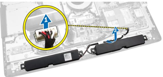
4. Remove the screws that secure the speakers to the chassis. Lift the speakers from the computer.
