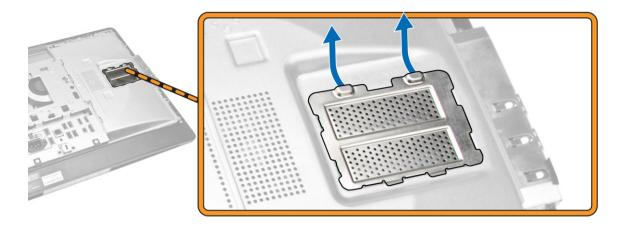
4. Pry the retention clips away from the memory module until it pops-up. Lift and remove the memory module from its connector.
