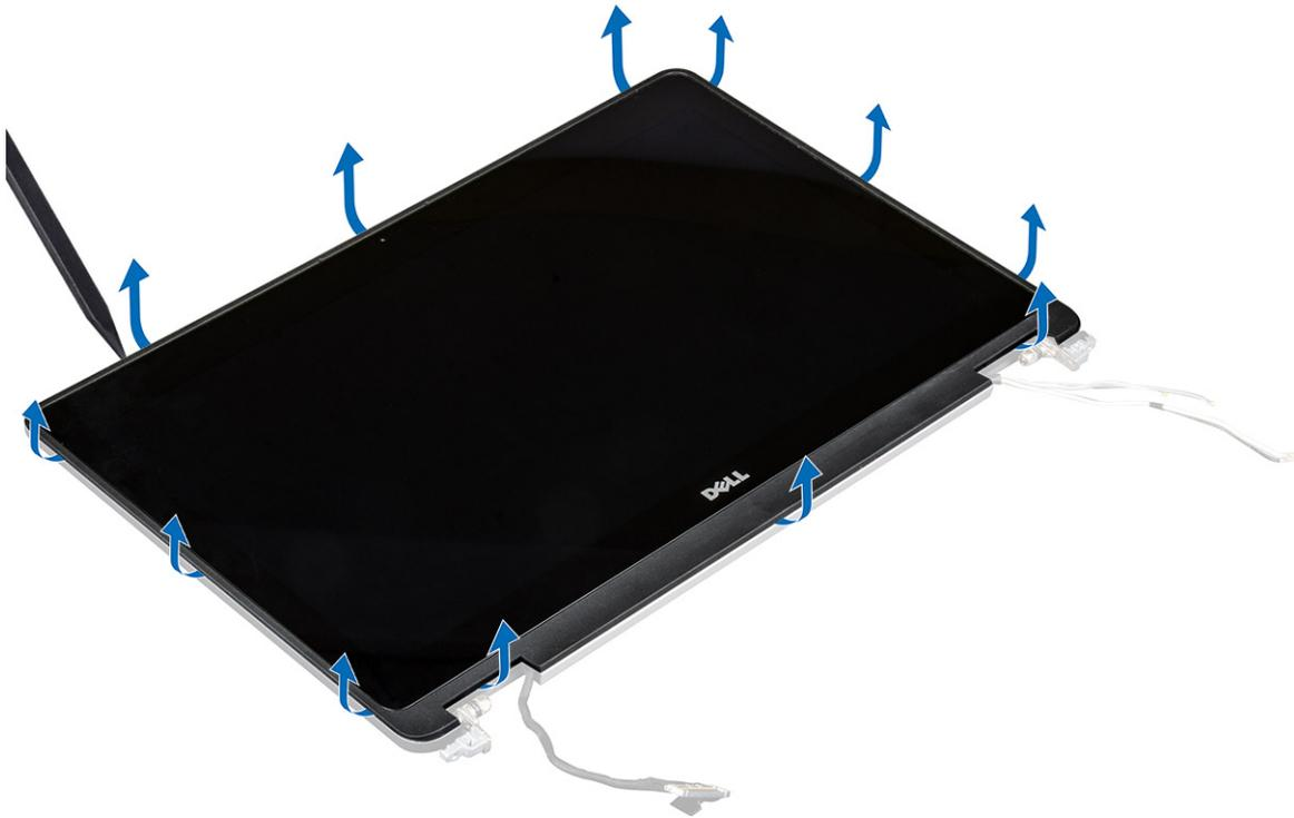
b Lift the display panel and turn the display panel over to access the eDP and display cables.
