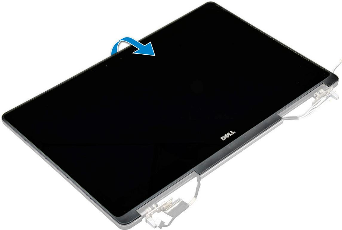
c Peel the adhesive to access the eDP cable [1, 5].
