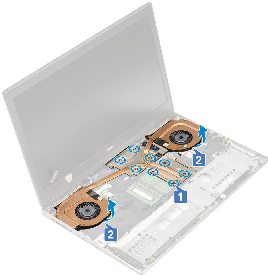
h. Slide and remove the heat sink assembly from the system.
