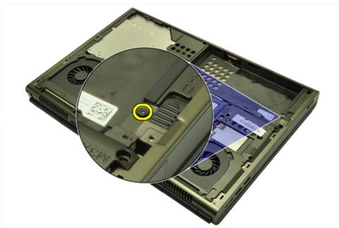
6. Slide the hard drive release latch into the unlock position.
