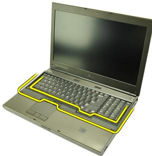
5. Lift up to remove the keyboard trim from the unit.
