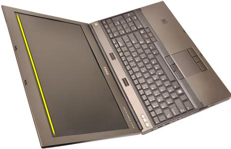
4. Work your way around the bottom edge and sides of the display bezel and remove the display bezel.
