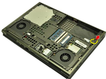
7. Remove the hard drive bracket from the system.
