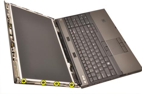
5. Remove the screws on the right side securing the display panel in place.
