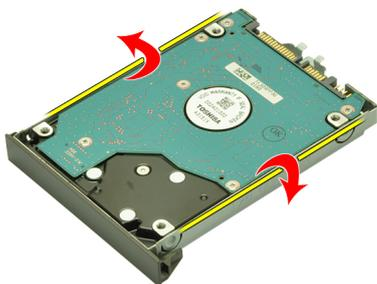
9. Remove the hard drive from the hard drive bracket.
