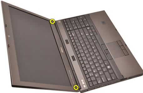
5. Carefully pry up the top edge of the display bezel.
