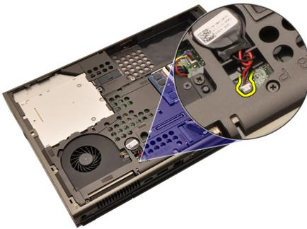
5. Pry up the coin—cell battery from the adhesive.
