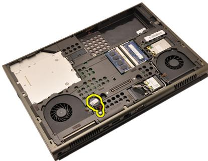
6. Remove the coin—cell battery from the system.
