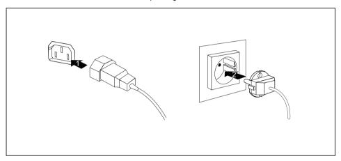
▶ Depending on your device configuration level, plug the monitor power cable into either the system unit (1) or a grounded mains outlet (2).
