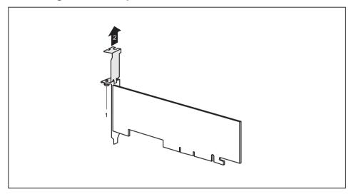
▶ Unscrew the screw (1) and remove the slot adapter (2).
