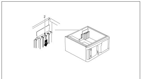
▶ Push the slot cover into the slot (1).
