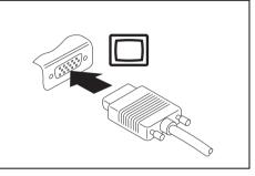
Analogue VGA monitor port (on the device and on the optional Port Replicator)
