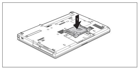
▶ Place the hard disk into the hard disk compartment (1).
