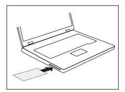
Slide the SmartCard into the SmartCard reader with the chip downwards and towards the front.
