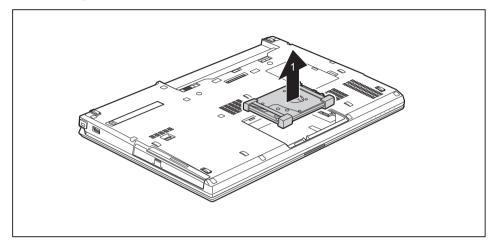
▶ Remove the hard disk from the hard disk compartment (1).
