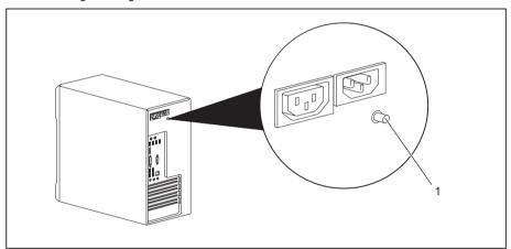
Press the emergency on button (1) to start the device.
