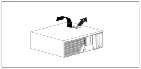
▶ Pull the locking device (1) and swivel the side part in the direction of the arrow (2).
