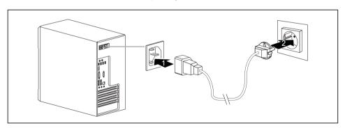
▶ Depending on your device configuration level, plug the monitor power cable into either the monitor socket of the device (1) or a grounded power outlet (2).
