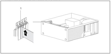
▶ Swivel the retaining clamp (1) around towards the back wall of the device.
