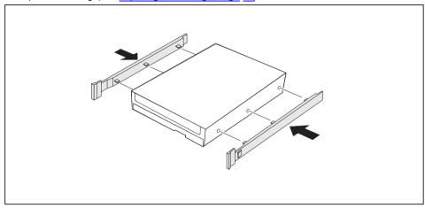
► Secure the EasyChange rails to the side of the hard disk drive by inserting the upper pins of the EasyChange rail in the corresponding holes of the hard disk.
