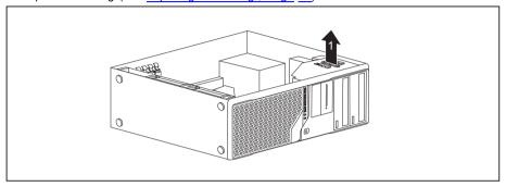
▶ Remove the drive cover from the bracket in the direction of the arrow (1).
