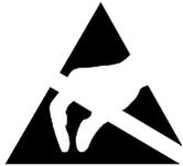
Boards with electrostatic sensitive devices (ESD) are marked with the label shown.
