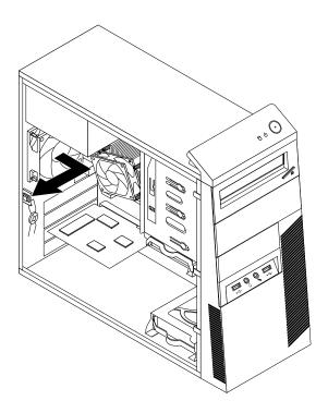
Figure 56. Removing the rear fan assembly
