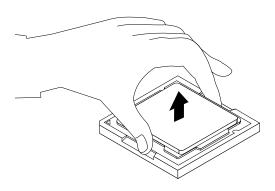
Figure 35. Removing the microprocessor
