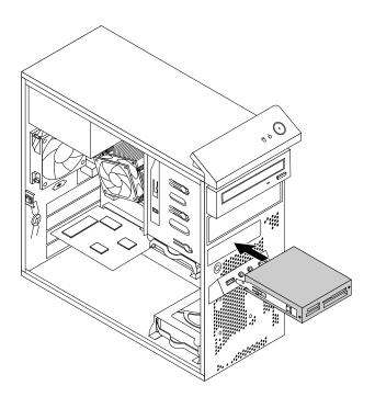
Figure 25. Installing the card reader
