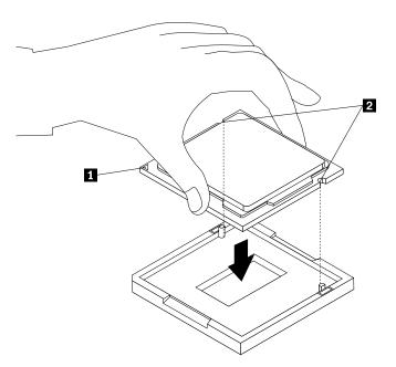
Figure 36. Installing the microprocessor
