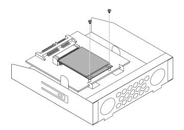
Figure 40. Installing the screws that secure the mSATA solid state drive
