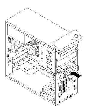
Figure 47. Installing the mSATA solid state drive
