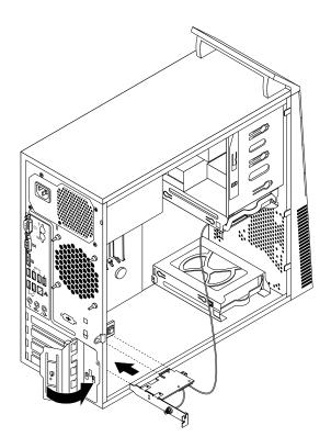
Figure 73. Installing the WiFi adapter card
