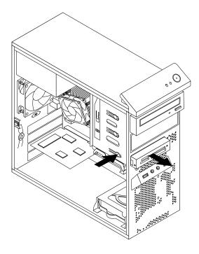
Figure 27. Removing the card reader
