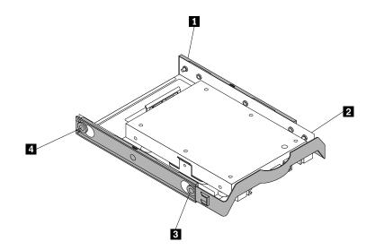
Figure 38. Installing the solid state drive with the storage converter into the hard disk drive bracket
