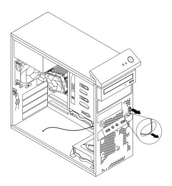
Figure 78. Removing the front WiFi antenna
