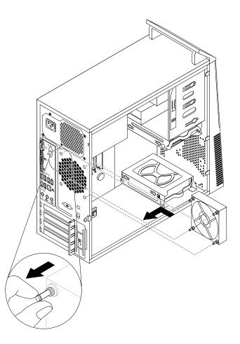
Figure 57. Installing the rear fan assembly
