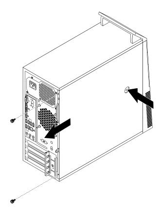
Figure 11. Removing the computer cover
