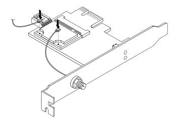
Figure 72. Installing the WiFi antenna cables
