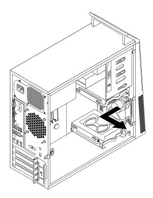
Figure 54. Removing the front fan assembly
