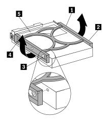
Figure 52. Installing the hard disk drive into the bracket
