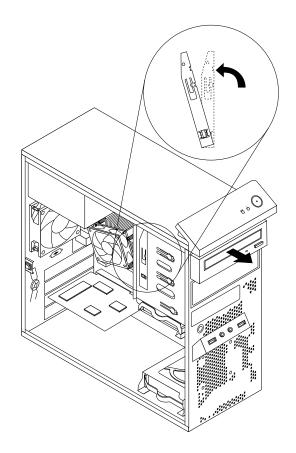
Figure 23. Removing the card reader retainer
