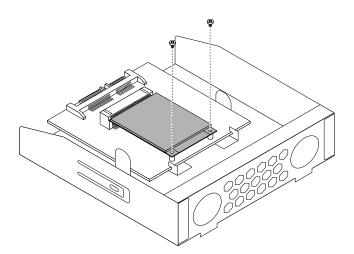
Figure 43. Removing the screws that secure the mSATA solid state drive
