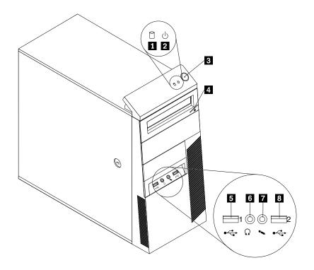
Figure 1. Front connector, control, and indicator locations
