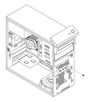
Figure 58. Removing the screw that secures the front audio and USB assembly to the chassis
