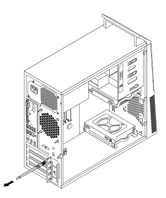
Figure 75. Removing the rear WiFi antenna
