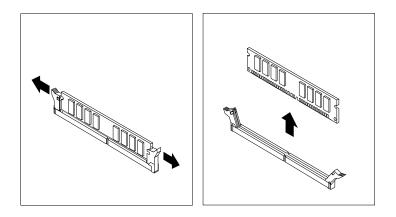
Figure 16. Removing a memory module
