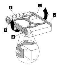
Figure 49. Installing the hard disk drive into the bracket
