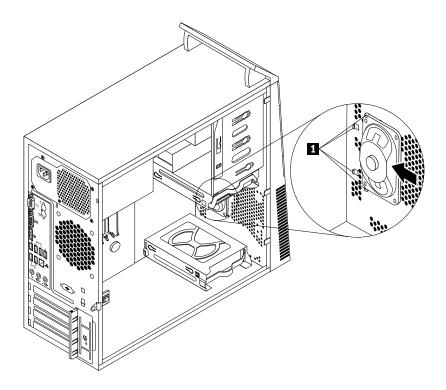
Figure 60. Installing a new internal speaker
