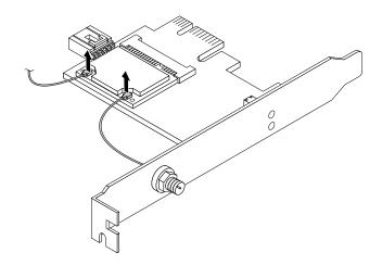
Figure 68. Removing the WiFi antenna cables
