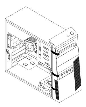
Figure 12. Removing the front bezel
