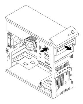
Figure 19. Removing the optical drive
