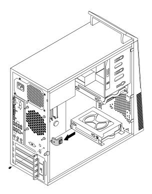
Figure 64. Installing the new cover presence switch
