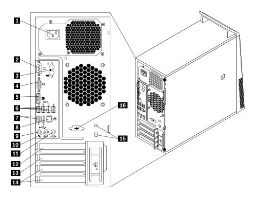
Figure 2. Rear connector locations
