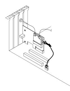
Figure 65. Disconnecting the Bluetooth cable
