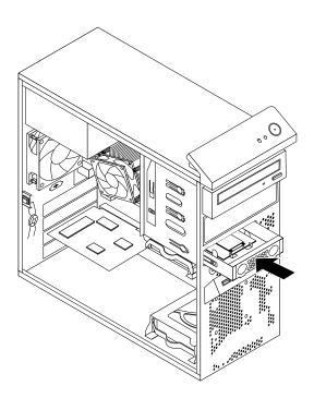
Figure 41. Installing the mSATA solid state drive
