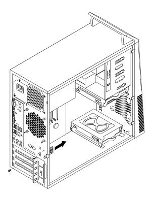
Figure 63. Removing the cover presence switch
