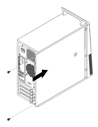
Figure 80. Reinstalling the computer cover
