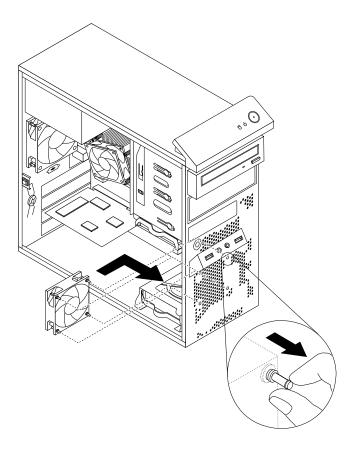
Figure 55. Installing the front fan assembly
