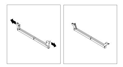
Figure 17. Opening the retaining clips
