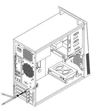
Figure 74. Installing the rear WiFi antenna
