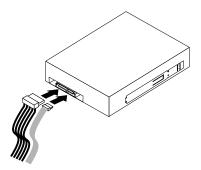
Figure 22. Connecting the optical drive
