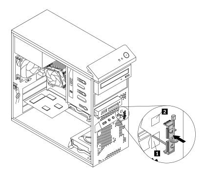
Figure 62. Installing the new thermal sensor
