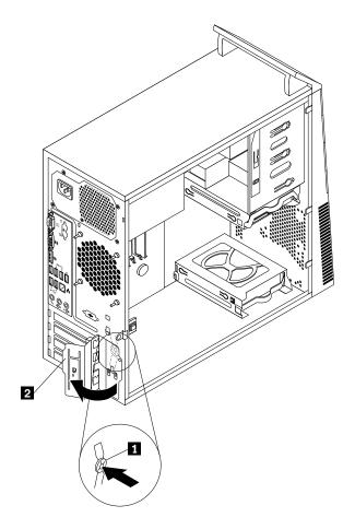
Figure 13. Opening the PCI card latch
