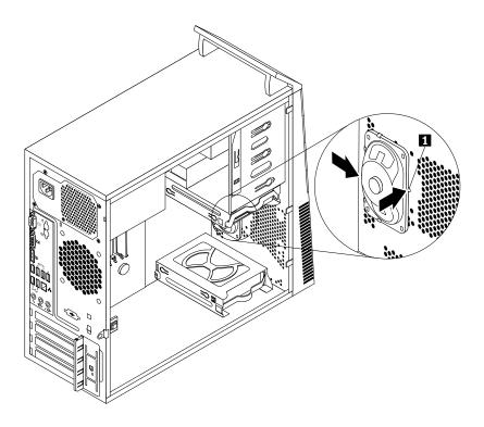
Figure 59. Removing the old internal speaker
