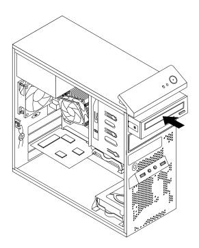
Figure 21. Installing the optical drive
