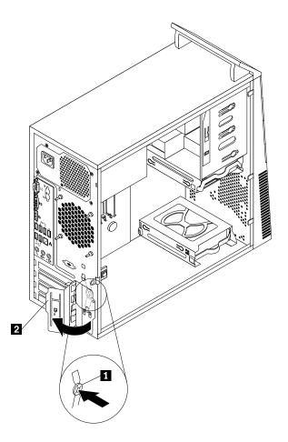
Figure 66. Opening the PCI card latch
