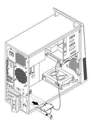
Figure 67. Removing the WiFi adapter card
