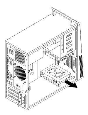
Figure 51. Removing the secondary hard disk drive
