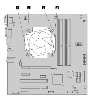
Figure 33. Removing the heat sink and fan assembly
