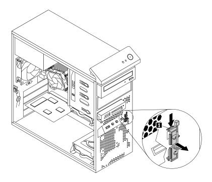
Figure 61. Removing the thermal sensor
