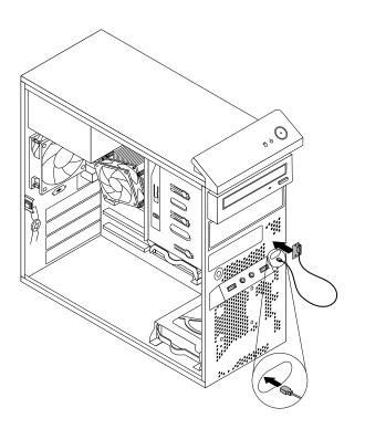
Figure 77. Installing the front WiFi antenna
