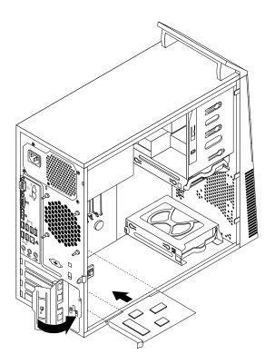
Figure 15. Installing a PCI card
