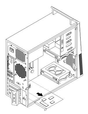
Figure 14. Removing a PCI card
