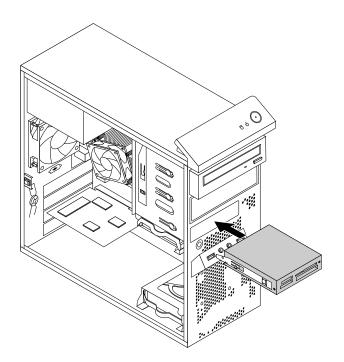
Figure 29. Installing the card reader
