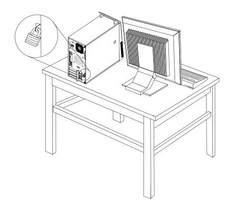
Figure 8. Installing a padlock
