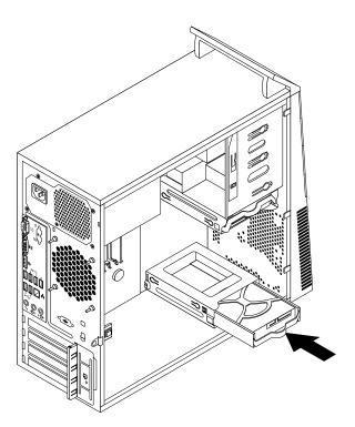
Figure 53. Installing the secondary hard disk drive
