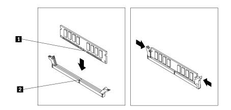
Figure 18. Installing a memory module
