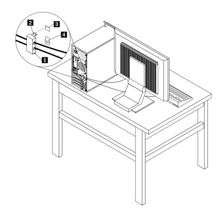
Figure 9. Installing a cable lock
