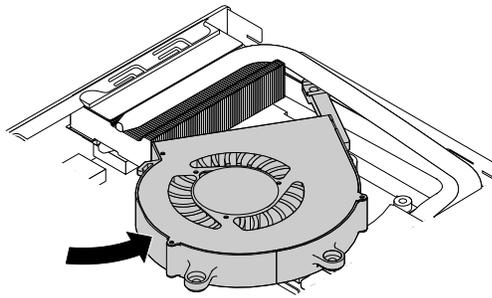
Figure 45. Installing the system fan (for M900x)
