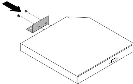
*Figure 21. Installing the external optical drive metal plate*
