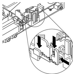
Figure 50. Securing the internal speaker cable
