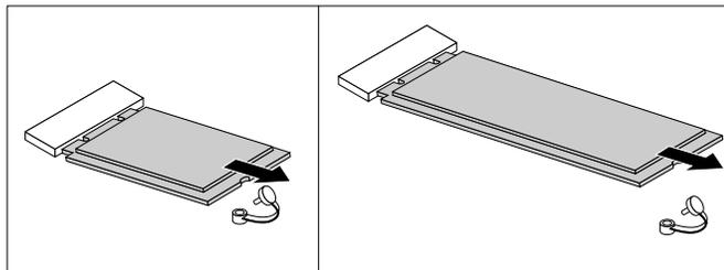
Figure 68. Removing the M.2 storage drive
