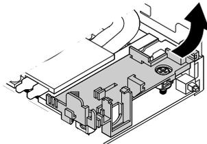
*Figure 52. Removing the internal speaker holder (for M900x)*
