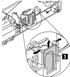
Figure 48. Removing the internal speaker
