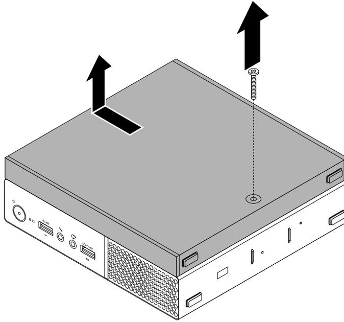
*Figure 18. Removing the external optical drive box*
