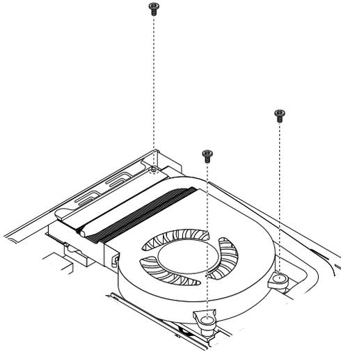
Figure 47. Installing the system fan screws (for M900x)
