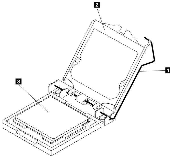
Figure 59. Opening the retainer to access the microprocessor
