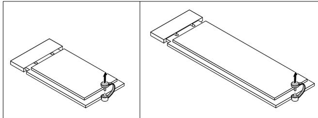
Figure 67. Removing the M.2 storage drive screw
