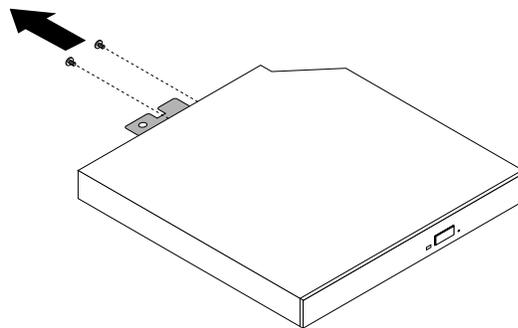
*Figure 20. Removing the external optical drive metal plate*
