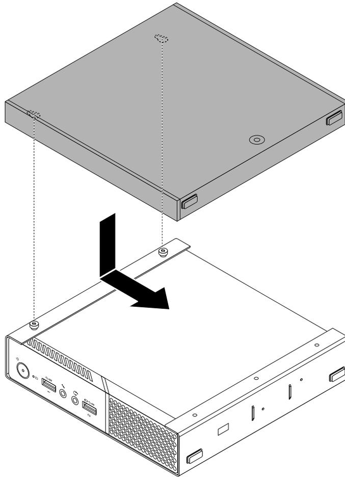
Figure 24. Installing the external optical drive box
