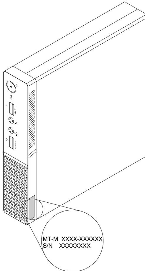
Figure 6. Machine type and model label
