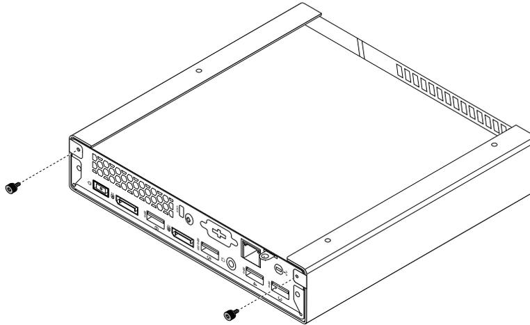
Figure 14. Removing the VESA mount bracket screws
