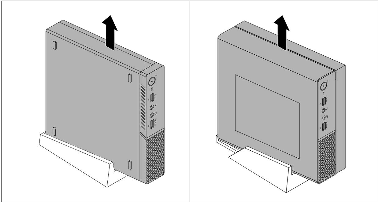
Figure 12. Removing the computer from the vertical stand
