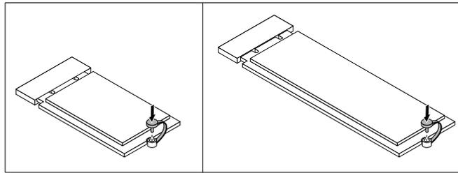
Figure 70. Installing the M.2 storage drive screw
