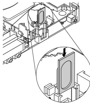
Figure 49. Installing the internal speaker
