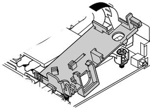
Figure 54. Installing the internal speaker holder (for M900x)
