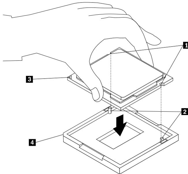
Figure 61. Installing the microprocessor
