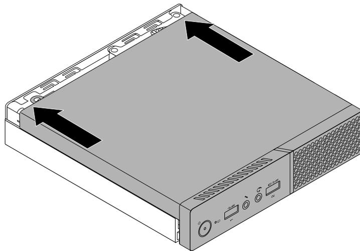
*Figure 87. Installing the computer cover*
