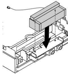
Figure 81. Sticking the front Wi-Fi antenna
