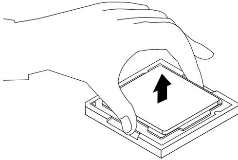
Figure 60. Removing the microprocessor
