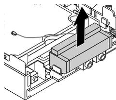
Figure 79. Removing the front Wi-Fi antenna
