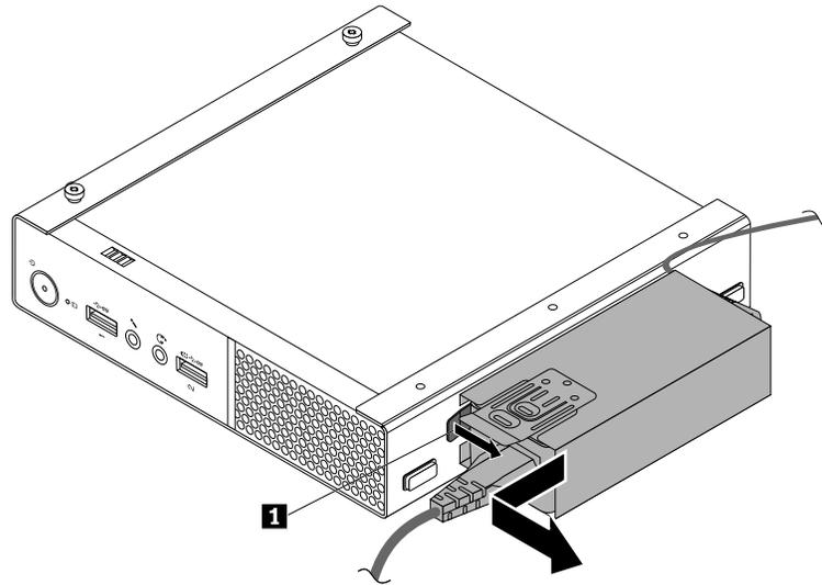
Figure 34. Removing the power adapter bracket
