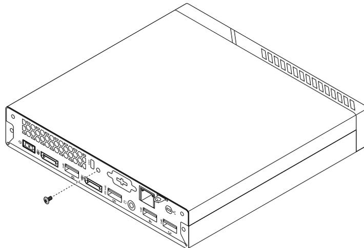
Figure 39. Removing the computer cover screw
