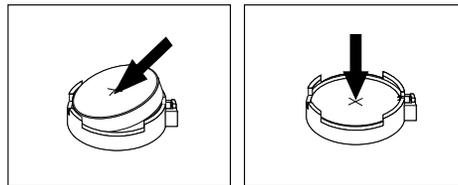
Figure 74. Installing the coin-cell battery
