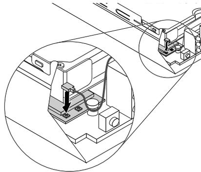
Figure 82. Installing the front Wi-Fi antenna cable
