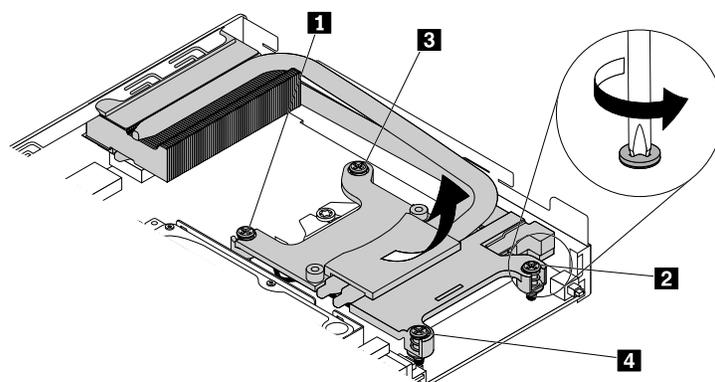
Figure 56. Removing the heat sink (for M900x)
