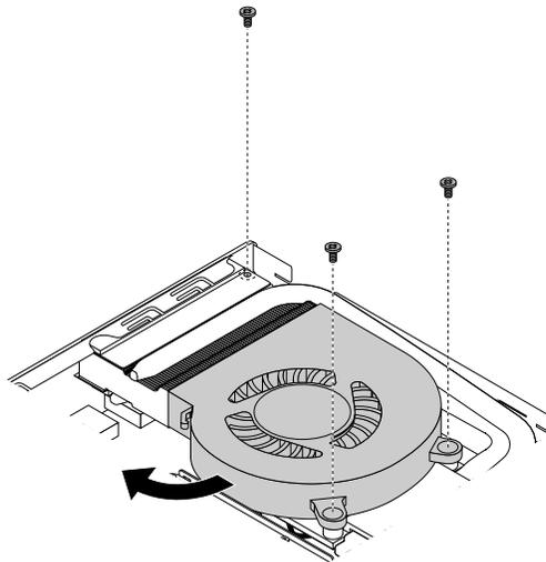
Figure 43. Removing the system fan (for M900x)
