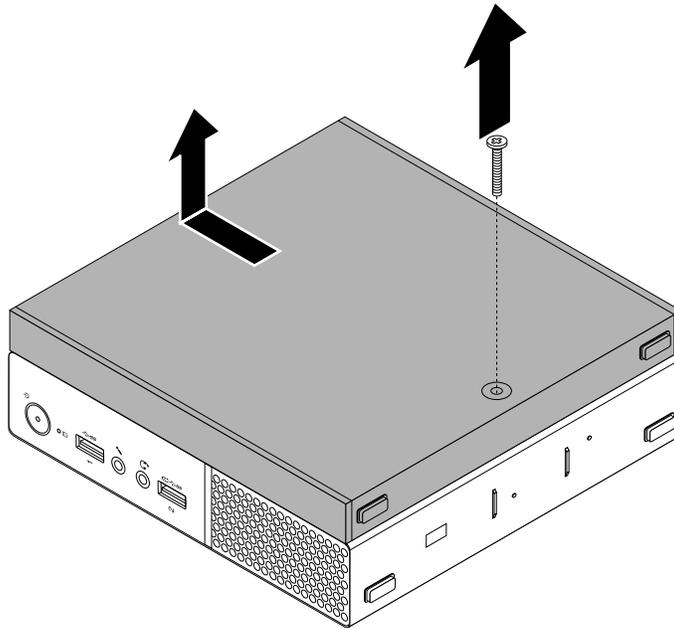
Figure 26. Removing the I/O box
