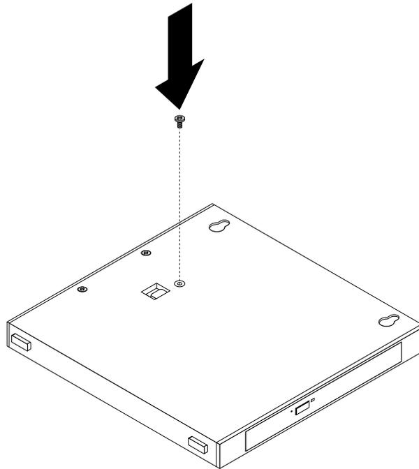
Figure 23. Installing the external optical drive screw
