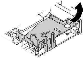
*Figure 51. Removing the internal speaker holder (for M700 and M900)*
