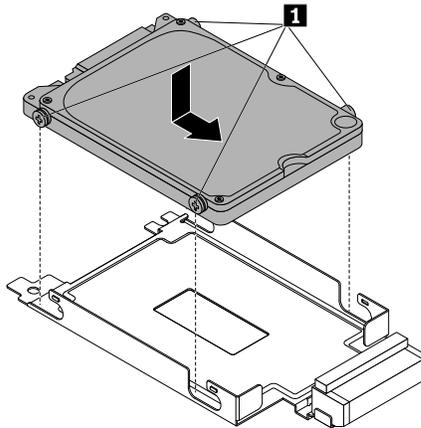
Figure 64. Installing the 2.5-inch storage drive
