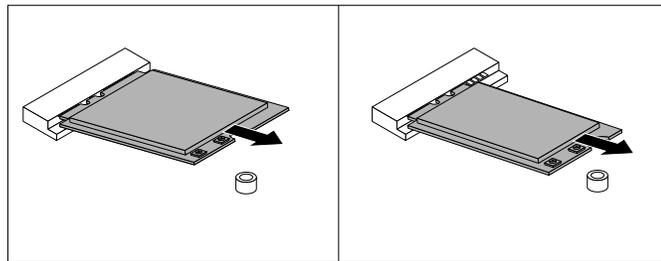
Figure 76. Removing the Wi-Fi card
