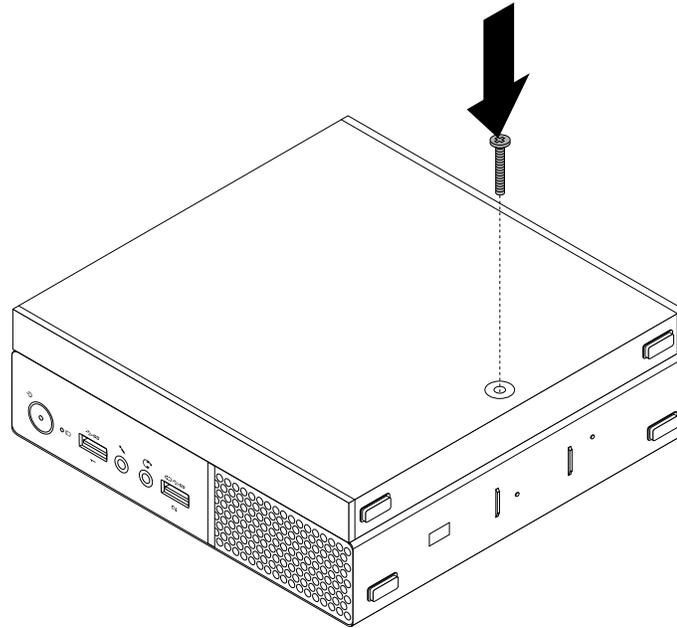
Figure 25. Installing the external optical drive box screw
