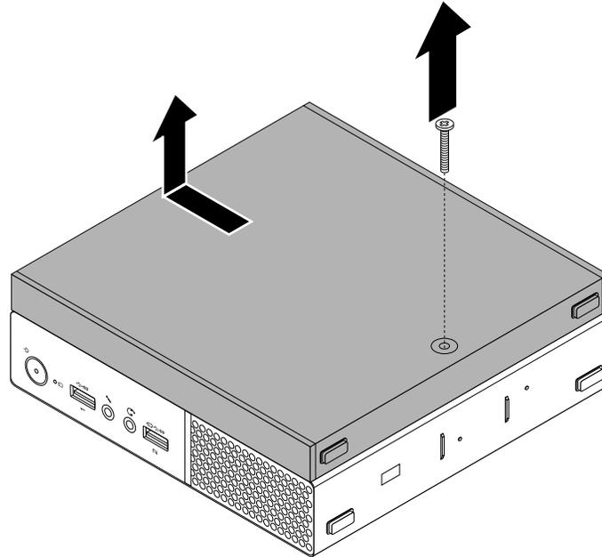
Figure 29. Removing the external battery box
