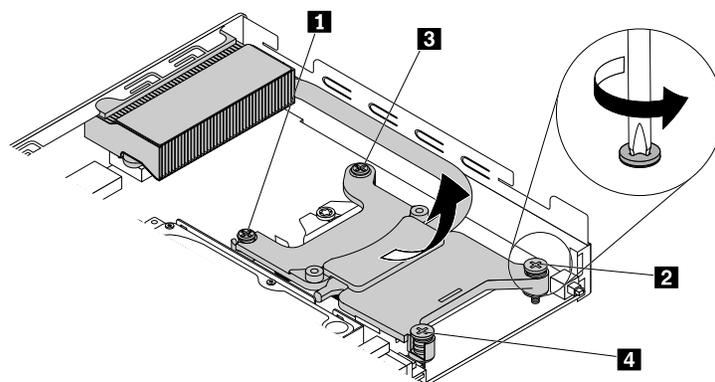
Figure 55. Removing the heat sink (for M700 and M900)
