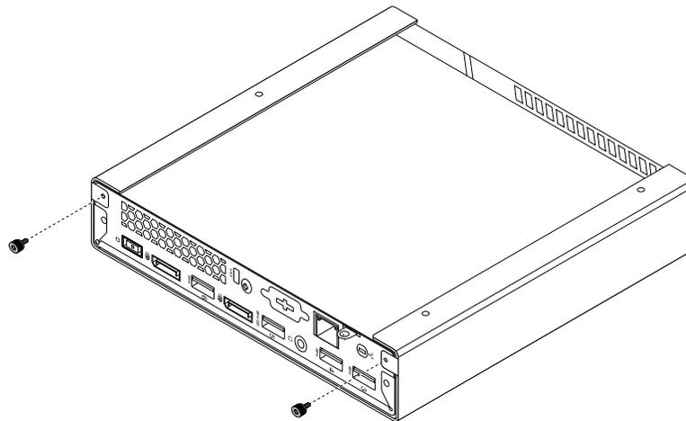
Figure 17. Installing the VESA mount bracket screws
