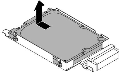
Figure 63. Removing the 2.5-inch storage drive
