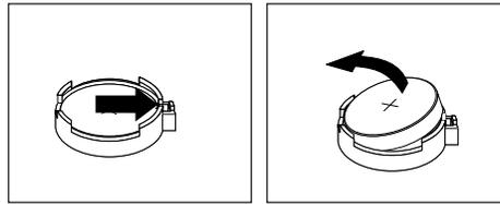
Figure 73. Removing the coin-cell battery
