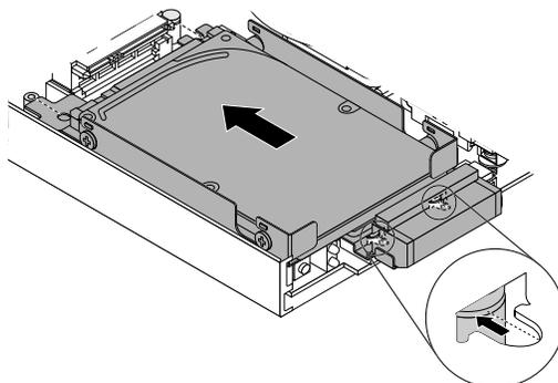
Figure 65. Installing the storage drive bracket
