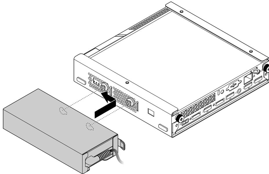
Figure 37. Installing the power adapter bracket
