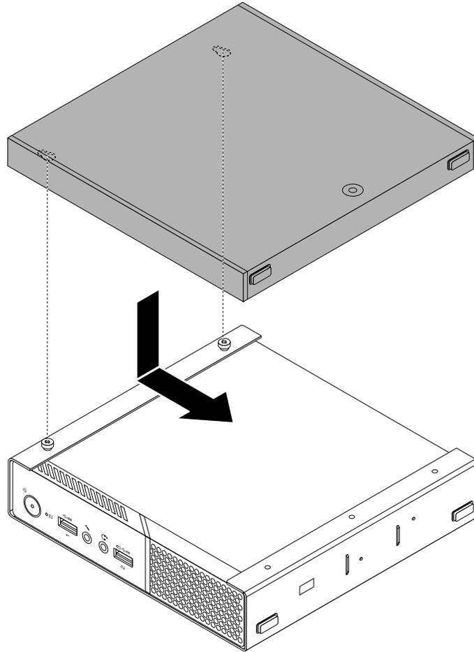
Figure 27. Installing the I/O box
