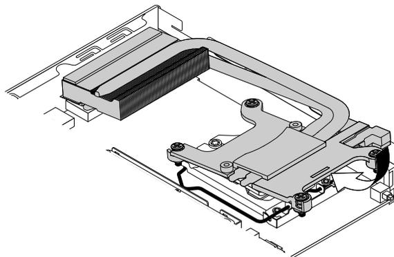
Figure 58. Installing the heat sink (for M900x)
