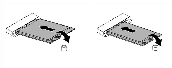
Figure 77. Installing the Wi-Fi card
