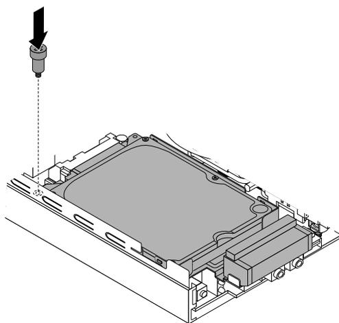
Figure 66. Installing the storage drive bracket screw
