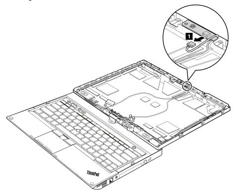
When installing: Ensure that the connector is attached firmly.
