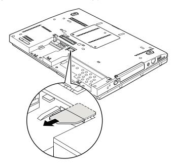
After you finish the servicing, ensure that you insert the card back into the slot firmly.
