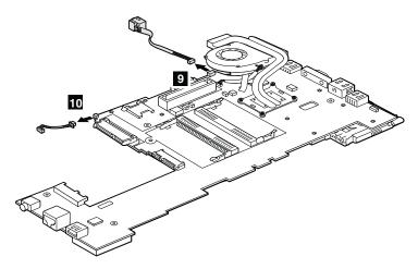
When installing: Ensure that the connectors are attached firmly to the system board.
