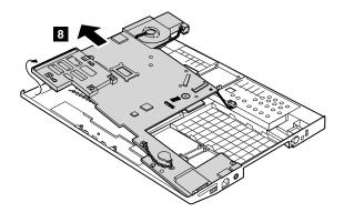
Disconnect the DC-in connector and the Tablet Digitizer Pen switch connector from the system board.
