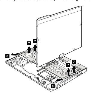
When installing: Ensure that all the latches are attached firmly.
