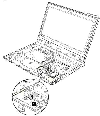
Unplug the connectors by using the antenna RF connector removal tool or pick the connectors with your fingers and gently unplug them in the direction shown by the arrow 2.
