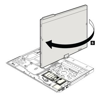
In step 7, detach the latches. Then remove the keyboard bezel in the direction shown by the arrow 8. Attention: When you service the keyboard bezel, avoid any kind of rough handling.
