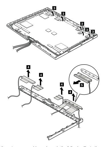
When installing: Place the antenna assembly as shown in the following illustration.
