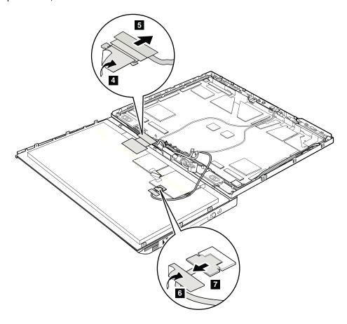
When installing: Ensure that the connectors are attached firmly.
