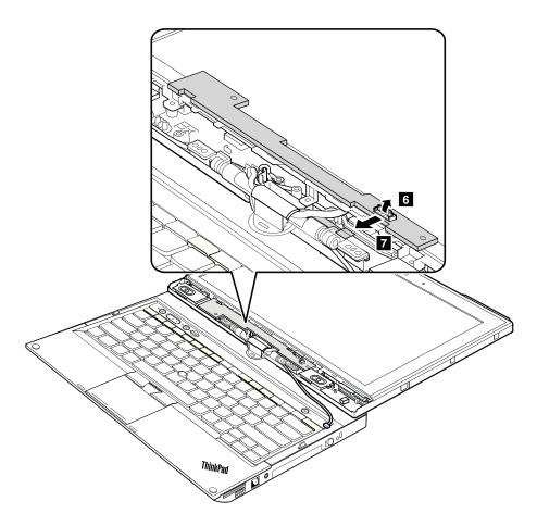
When installing: Ensure that the connector is attached firmly.
