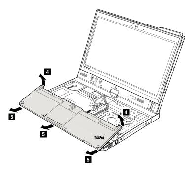
**When installing:** Press the front edge of the palm rest to fit it into place **1**. Then, press the rear edge of the palm rest until it clicks into place **2**.
