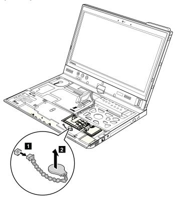
When installing: Ensure that the battery connector is attached firmly.
