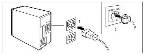
Depending on your device configuration level, plug the monitor power cable into either the PC (1) or the grounded mains outlet (2).
