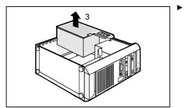
Carefully pull the power supply out of the casing (3).
