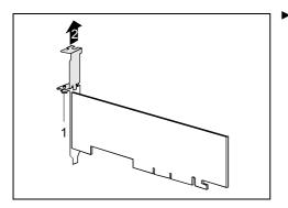
Unscrew the screw (1) and remove the slot adapter (2).
