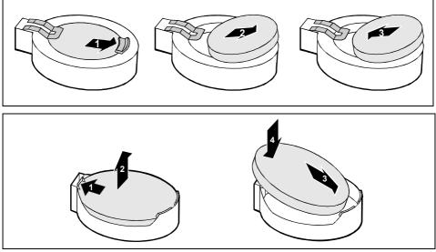
The lithium battery holder exists in different designs that function in the same way.
