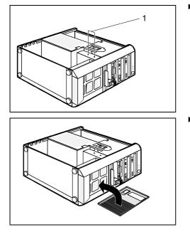
Secure the WLAN module with the two screws (1) provided.
