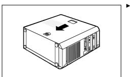
Push the top cover down in the direction of the arrow (1) until it engages.
