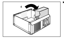
Tilt and turn the power supply unit so that it engages in the mounting on the front casing (4).
