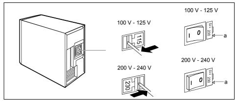
a = Notch for inserting the screwdriver
