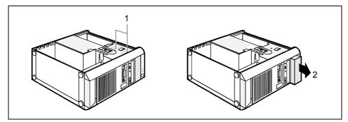
Remove the screws (1) and take the blind insert out of the casing (2).
