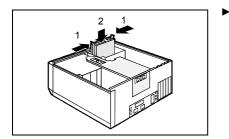
Secure the EasyChange rails on the side of the hard disk by inserting the upper pins of the EasyChange rail in the corresponding holes of the hard disk.
