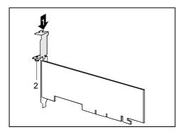
► Fit the slot adapter on the slot cover of the low-profile board (1) and screw it on (2).
