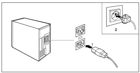
Connect the power cable first to the PC (1) and then to the grounded mains outlet (2).
