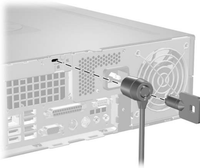
Figure C-1 Installing a Cable Lock
