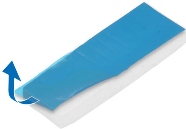
3. Place the rubber on the computer [1] and peel the adhesive tape (pink) from the rubber [2].
