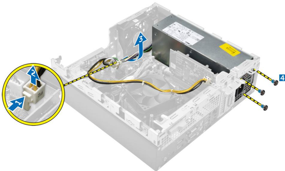
5. Press the blue release tab [1], slide the PSU and lift it away from the computer [2].
