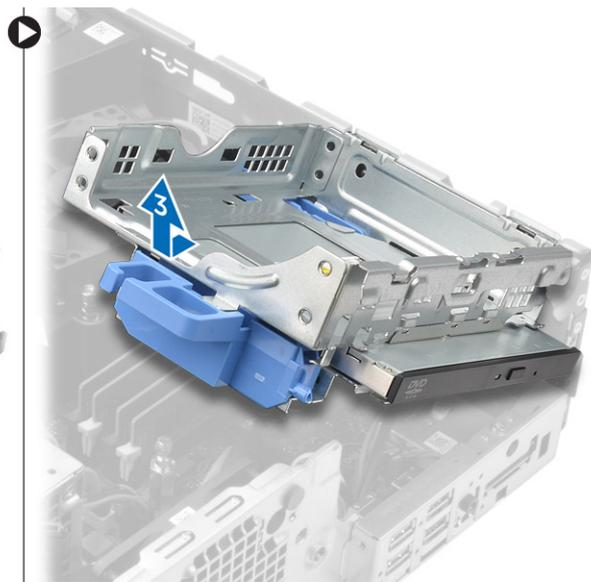
5. To remove the optical drive from the optical drive cage:
