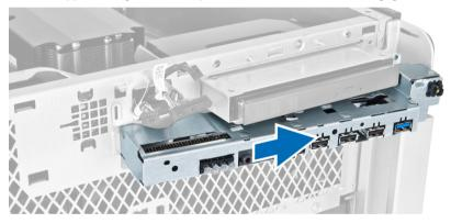
Remove the screws that secure the USB 3.0 module to the I/O panel assembly and remove it from the computer.
