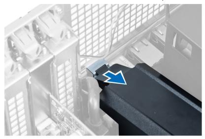
5 Press down on the release latch on the memory shroud base and lift it upwards to remove it from the computer.
