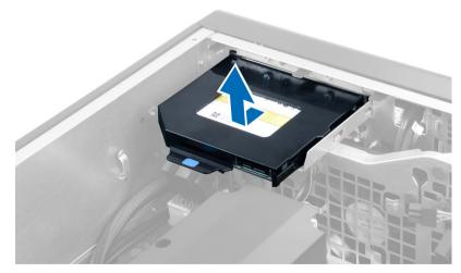
7 Flex the optical-drive bracket latches in an outward direction to loosen the optical drive from the bracket.
