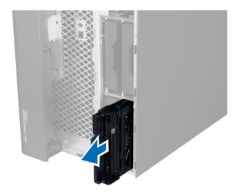
5 If a second hard drive is installed, Pull the clasp of the second hard-drive bracket in an outward direction.
