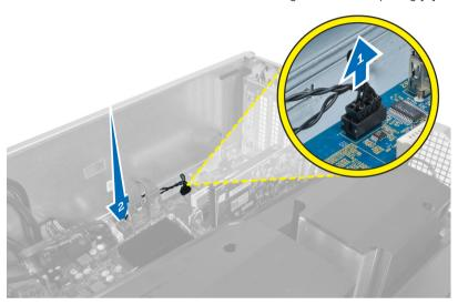
4 Unroute the HDD thermal-sensor cable from its securing clips on the chassis.
