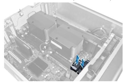
6 Repeat the steps to remove the second memory shroud module and memory shroud base from the computer.
