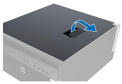
3 Lift the cover upward to a 45-degree angle and remove it from the computer.
