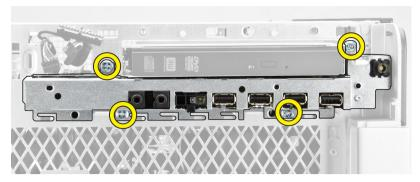
5 Pull the I/O panel assembly in a direction opposite to the computer to release its edge from the chassis clip.
