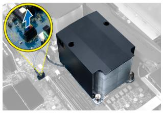
4 Remove the captive screws that secure the heatsink.
