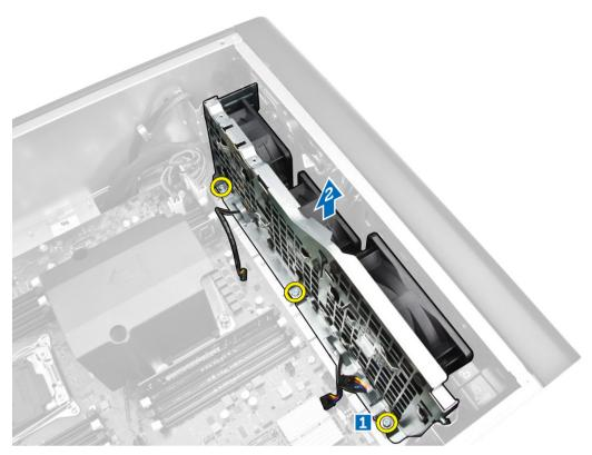
10 Insert the fan cable through the opening to release the system-fan module.
