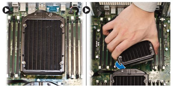
4 Remove the heatsink fan cable from the system board.
