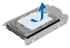
9 If a 2.5 inch hard drive is installed, Push the retention clips in an outward direction and lift up the drive to remove it from the 3.5 inch hard-drive caddy.
