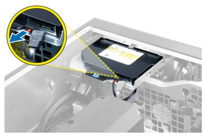
5 Pull up the blue release tab to release the latches that secure the optical drive.
