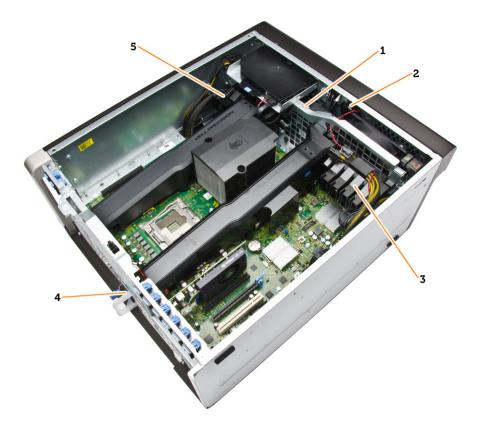
Figure 3. Inside View of T7910 Computer
