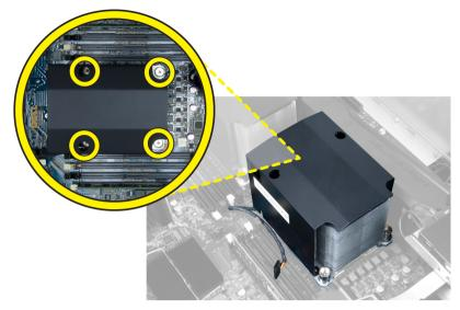
5 Lift up the heatsink and remove it from the computer.
