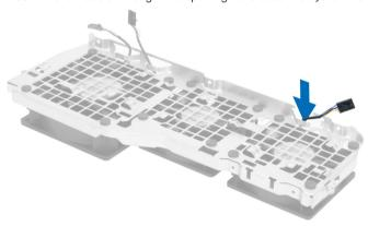
11 Remove the grommets that secure the system fan , lift up the fan and remove it from the fan assembly.
