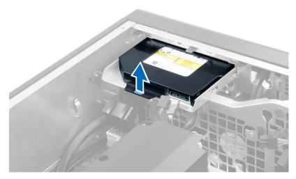
6 Slide the optical drive out of its compartment and lift it up to remove it from the computer.
