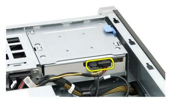
4 Press the release latch and slide the optical drive outward to release it from the drive bay [1, 2].
