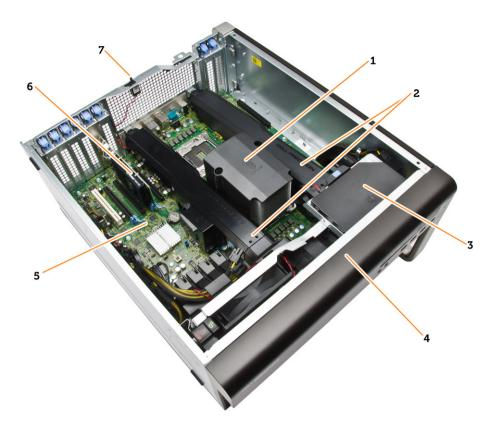
Figure 2. Inside View of T7910 Computer
