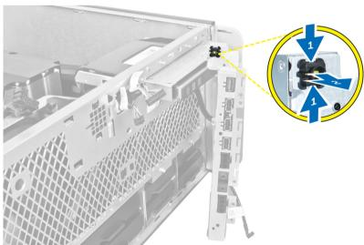
Remove the power switch from the computer.
