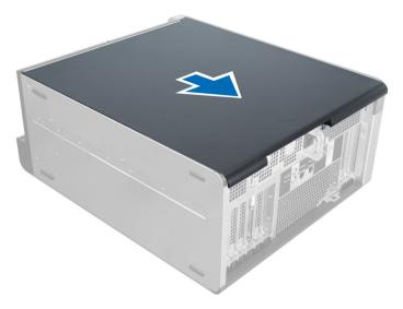
4 Lift the right cover at a 45-degree and remove it from the computer.
