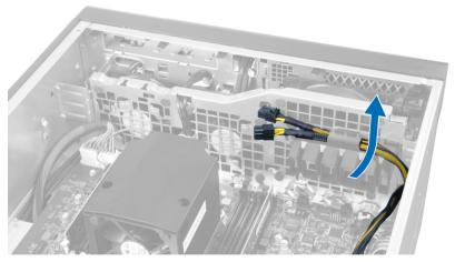
7 Route the system-fan cable through the opening in the system-fan module.
