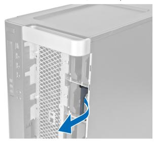
6 Slide the second hard-drive bracket in an outward direction to remove it from the computer.
