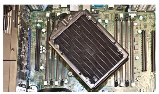
4 Connect the heatsink fan cable to the system board.
