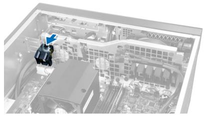
5 Lift the PCle card retention in an upward direction to remove it from the computer.
