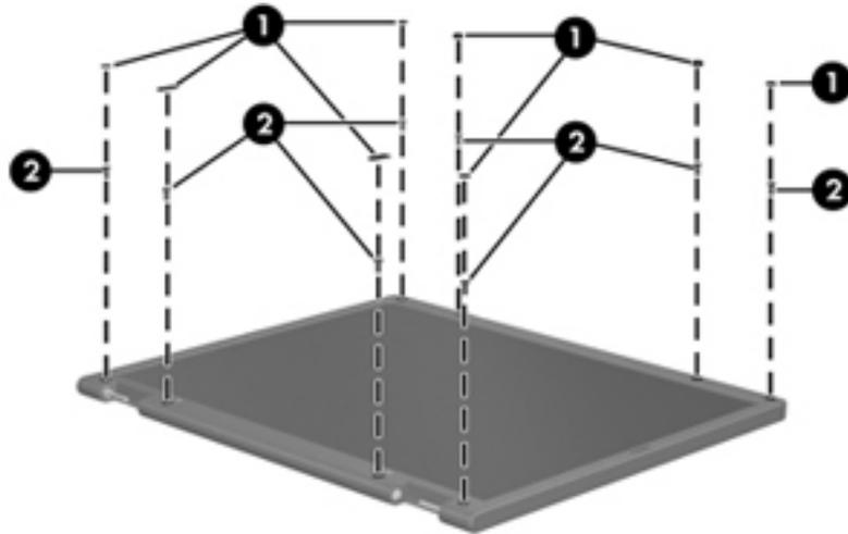
2. Lift up and out on the left and right inside edges ① and the top and bottom inside edges ② of the display bezel until the bezel disengages from the display assembly.
