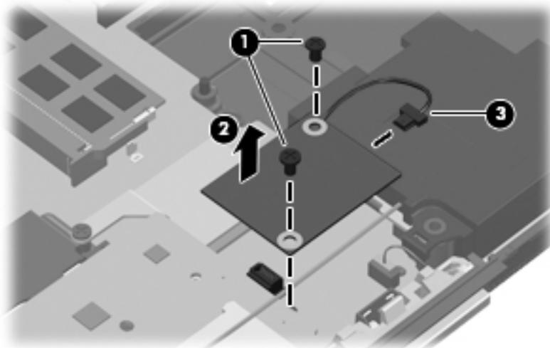
Reverse this procedure to install the modem module.
