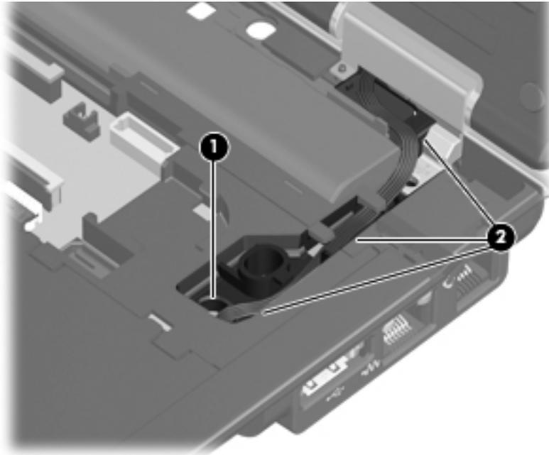
4. Disconnect to microphone cable ❶ from the system board.
