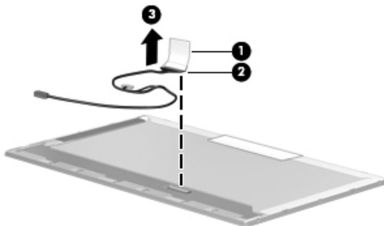
16. If necessary to replace the webcam module and cables, the dual-array microphone and microphone cable, or the wireless antennas and cables, replace the display back cover using the following part numbers:
