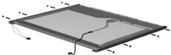
9. Use a sharp-edged tool to cut the tape ❶ that secures the sides of the display panel to the display panel frame.
