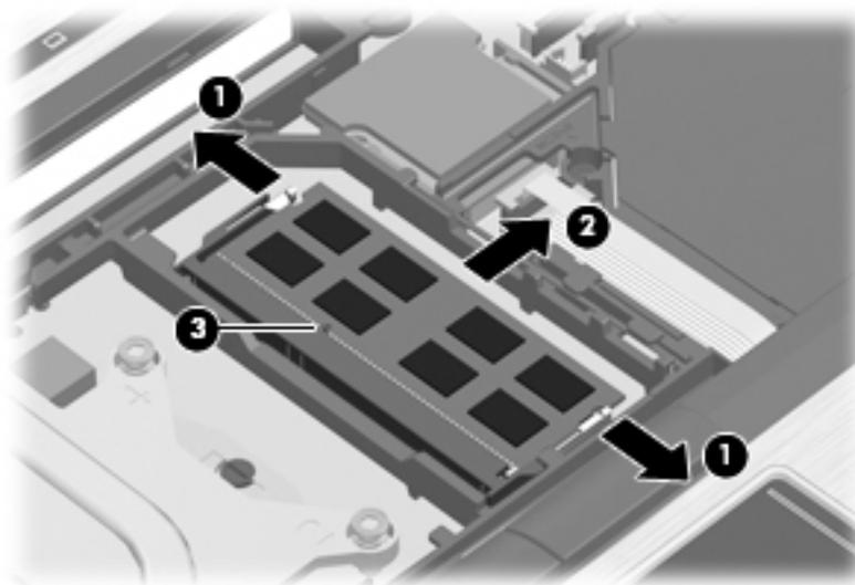
Reverse this procedure to install a primary memory module.
