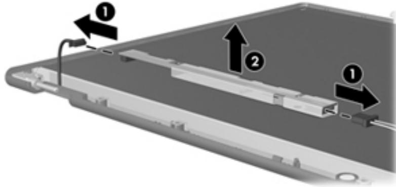
5. Remove all screws ❶ that secure the display panel assembly to the display enclosure.
