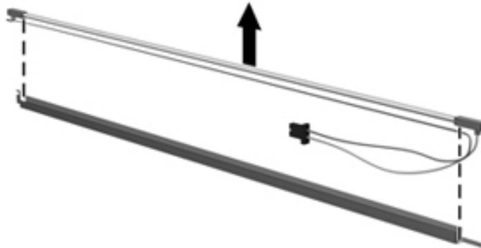
19. Disconnect the display cable ❶ from the LCD panel.
