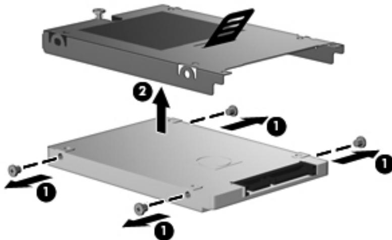
Reverse this procedure to reassemble and install the hard drive.
