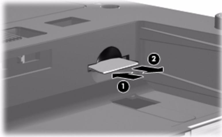
Install the SIM by inserting it into the SIM slot and pushing until you hear a click.
