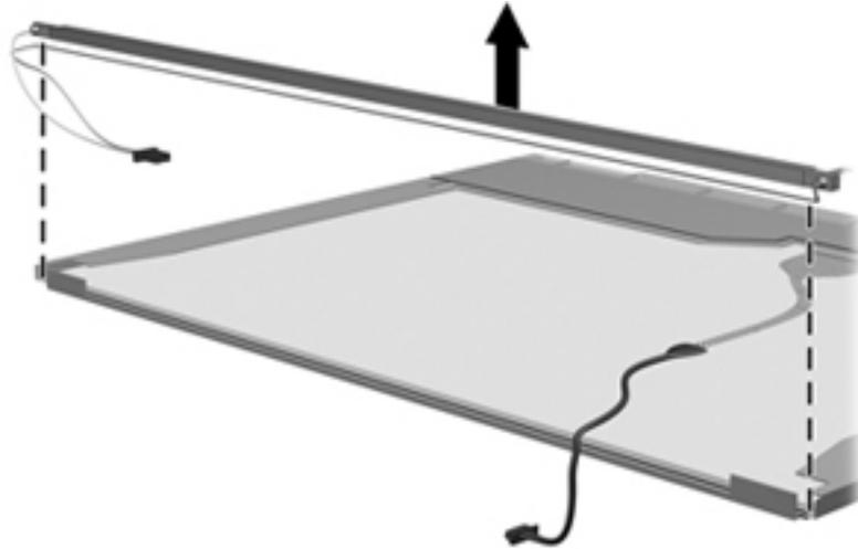
18. Remove the backlight from the backlight frame.
