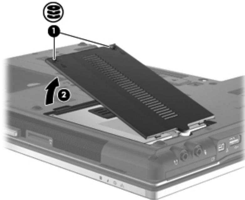
5. Loosen the Phillips PM2.5×10.0 captive screw ❶ that secures the hard drive to the computer.
