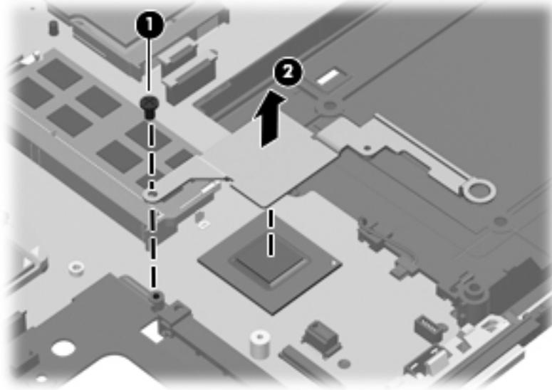
3. Remove the 2 Phillips PM2.5×4.0 screws ❶ that secure the system board to the base enclosure.
