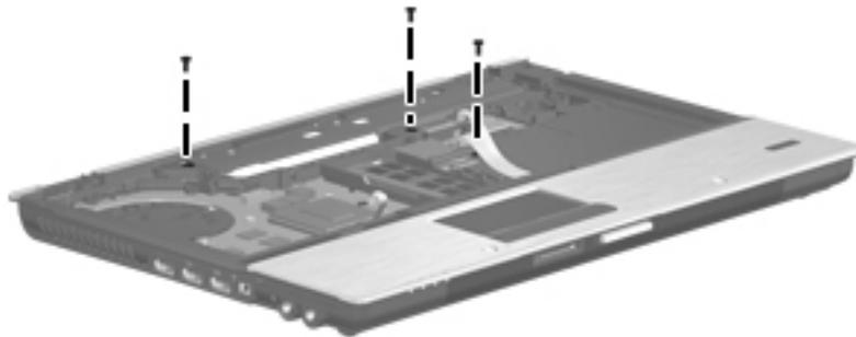
6. Lift the rear edge ❶ of the top cover until it detaches from the base enclosure.
