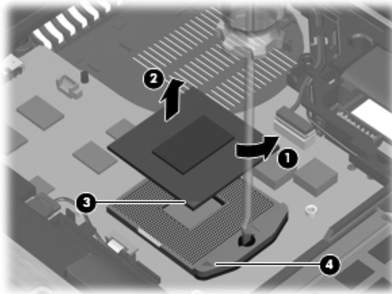
Clean and replace any thermal material, and then reverse this procedure to install the processor.
