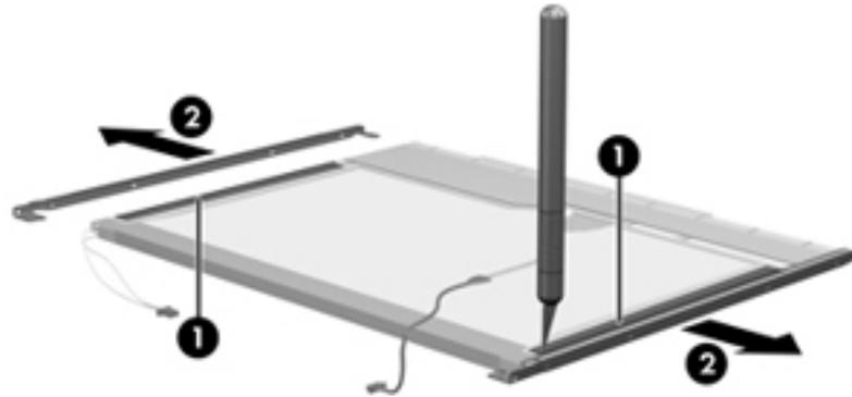
11. Remove the screws ❶ that secure the backlight cover to the display panel.
