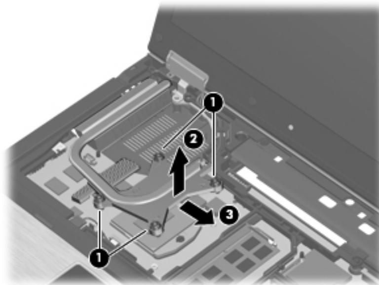
3. Remove the heat sink assembly.
