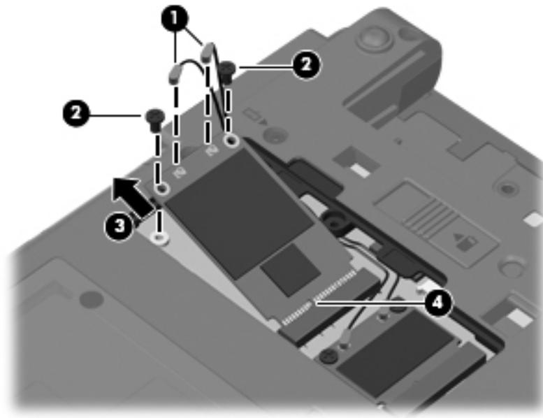
Reverse this procedure to install the WWAN module.
