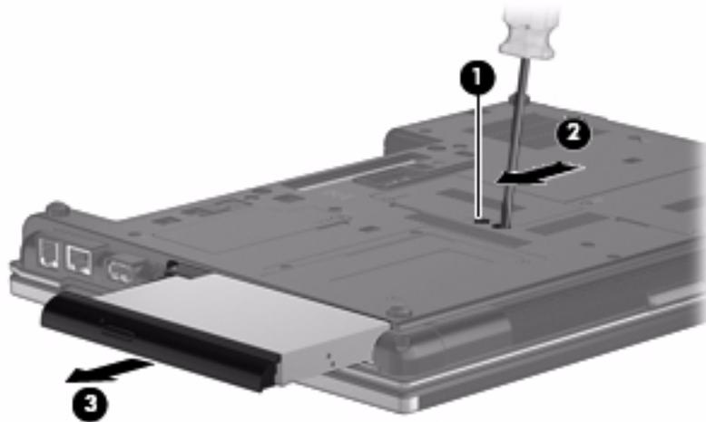
4. If it is necessary to replace the optical drive bracket, follow these steps:
