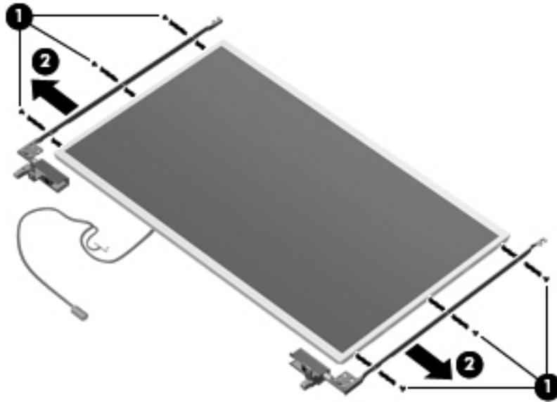
14. If it is necessary to replace the display hinge covers:
