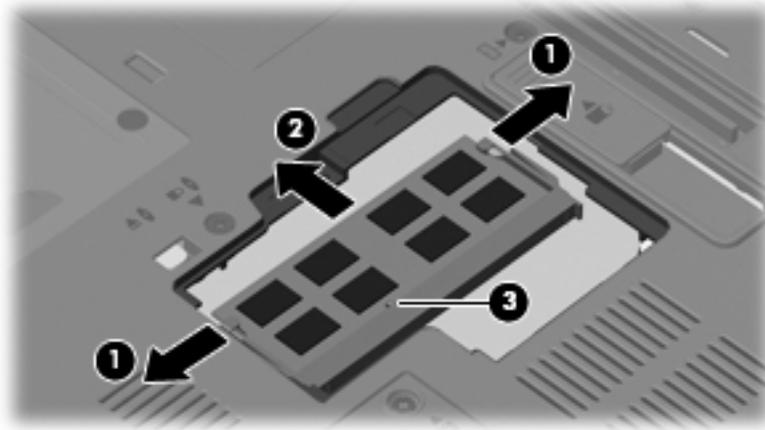
Reverse this procedure to install an expansion memory module.
