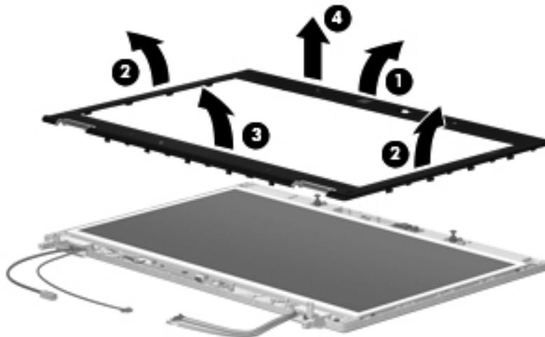
13. If it is necessary to replace the display hinges:
