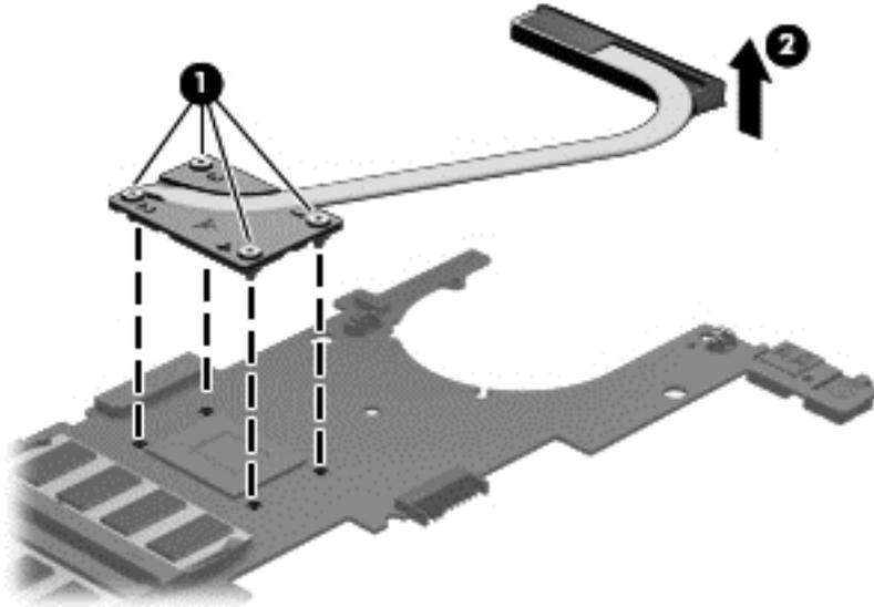
**NOTE:** The thermal material must be thoroughly cleaned from the surfaces of the heat sink and the system board components each time the heat sink is removed. Replacement thermal material is included with the heat sink, processor, and system board spare part kits.
