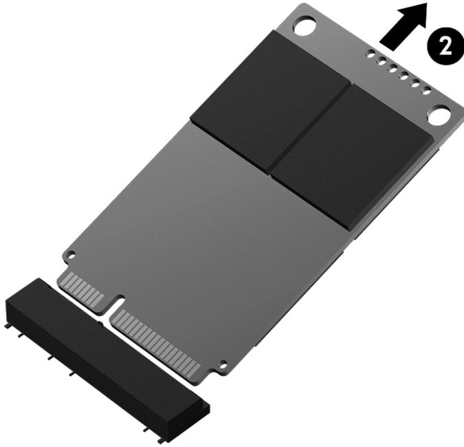
Reverse this procedure to install the mSATA drive.
