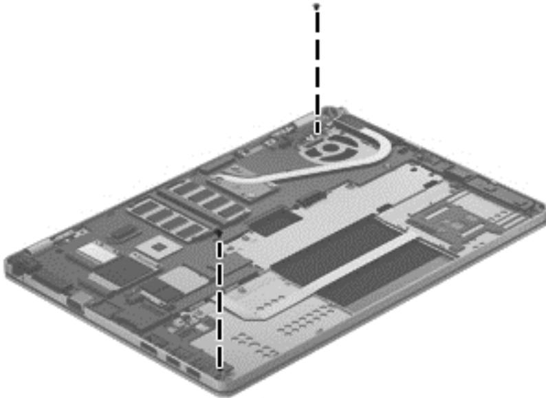
3. Lift the left side of the system board up at an angle **(1)**.
