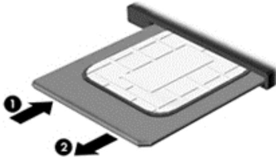
Reverse this procedure to install the SIM.
