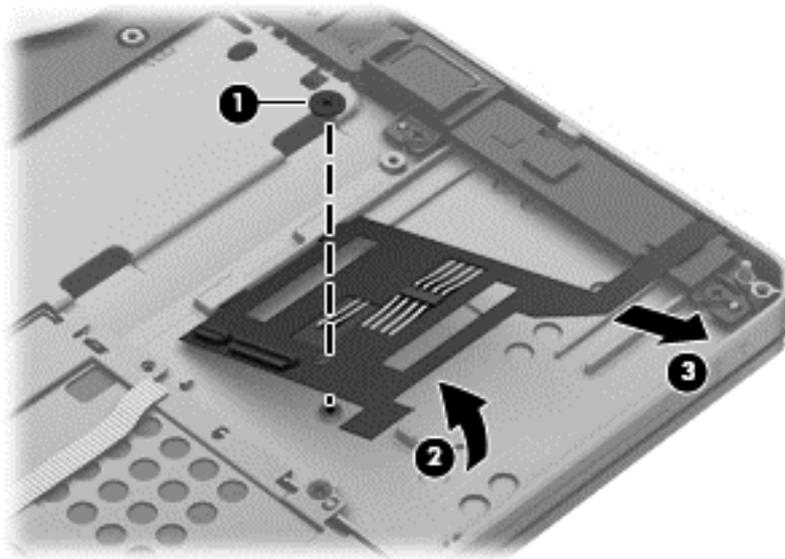
Reverse the removal procedures to install the smart card board.
