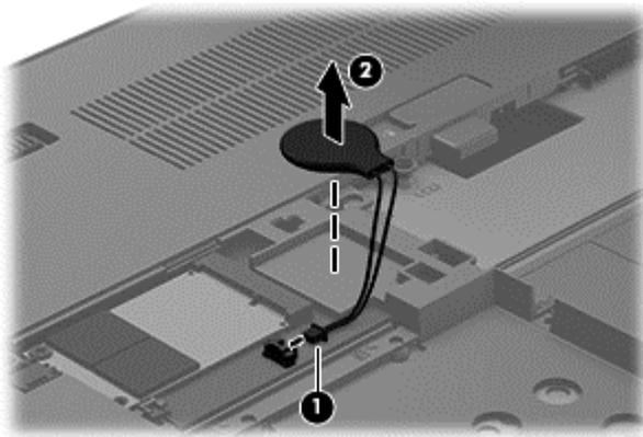
3. Remove the RTC battery.
