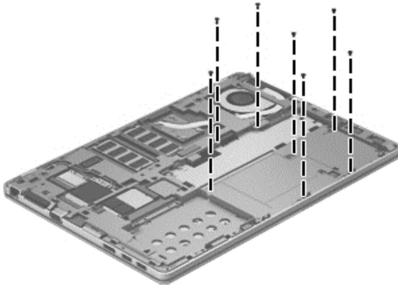
5. Lift the base enclosure **(1)** off the computer while threading the antenna cables through the hole in the base enclosure **(2)**.
