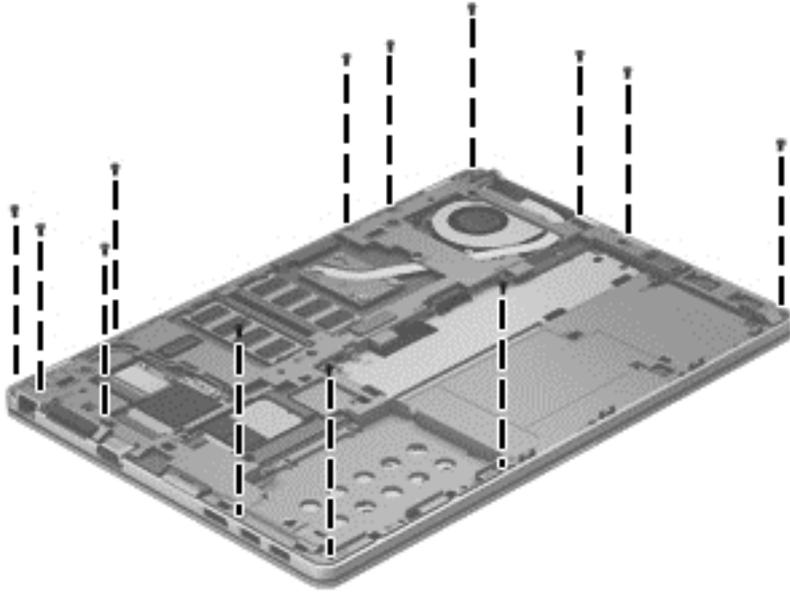
4. Remove the 7 Torx PM2.0×3.0 screws from the battery bay that secure the base enclosure to the computer.
