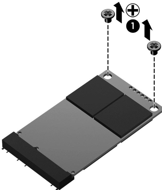
2. Remove the drive **(2)** by pulling it away from the slot at an angle.
