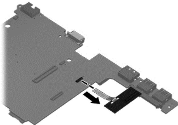
3. Remove the fingerprint reader board and cable.
