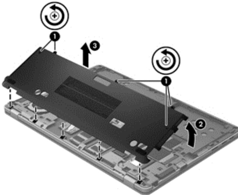
Reverse the removal procedures to install the service cover.
