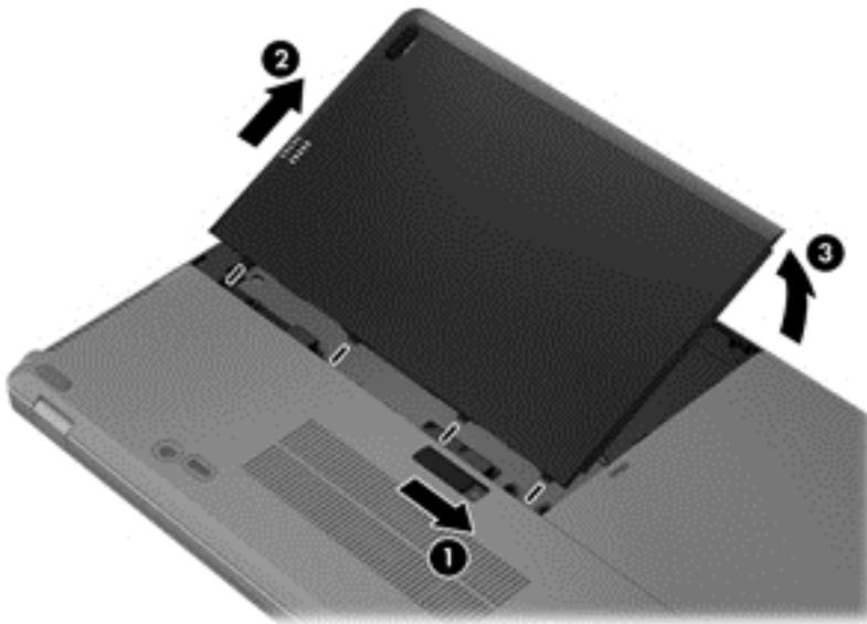
When installing the battery:
