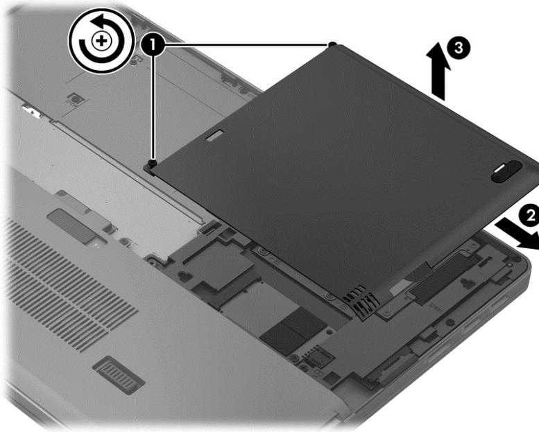
Reverse the removal procedures to install the hard drive cover.
