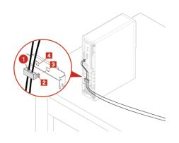
A cable lock can be used to secure devices, such as the keyboard and the mouse, by locking the device cables to the computer. The cable lock connects to the cable-lock slots on the rear of the computer.
