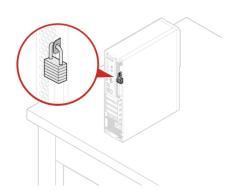
Locking the computer cover helps prevent unauthorized access to the inside of your computer. Your computer features a padlock loop so that the computer cover cannot be removed when a padlock is installed.
