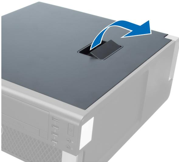
4. Lift the cover upward to a 45-degree angle, and remove it from the computer.
