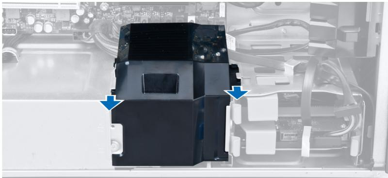
4. Remove the baffle cover from the computer.
