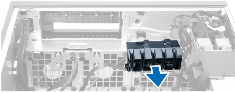
10. Disconnect the system-fan cables from the system board.
