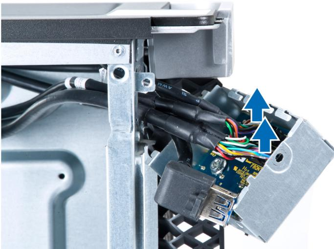
6. Remove the screws which secure the I/O panel to the chassis.
