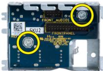
7. Remove the I/O panel from the chassis.
