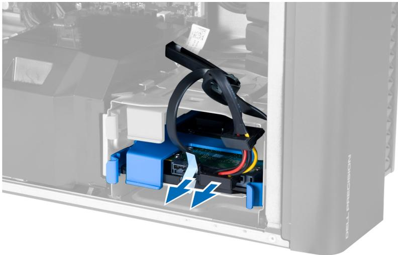
4. Press in on the latches on either side of the hard-drive bracket.
