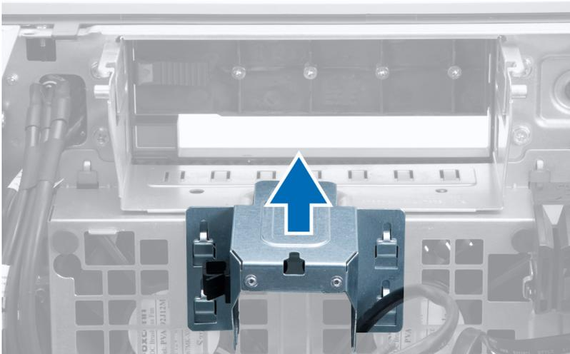
7. Remove the screws that secure the drive bay.
