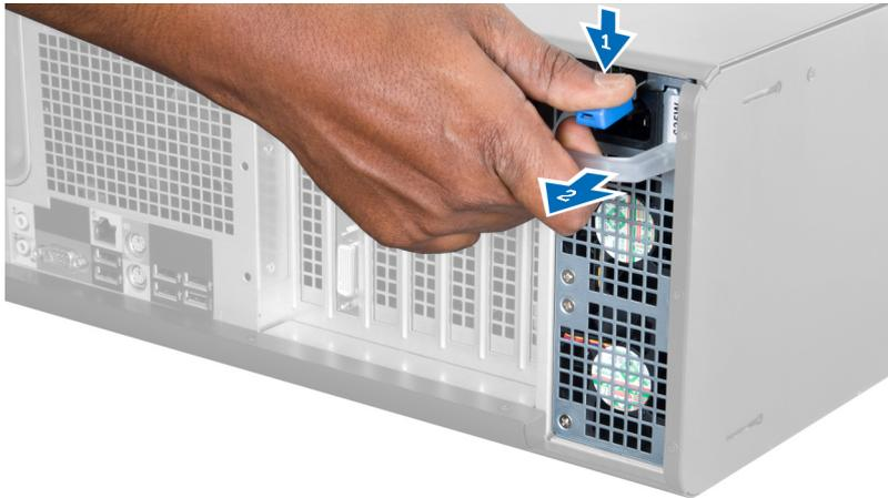
4. Hold the handle bar to slide the PSU out of the computer.
