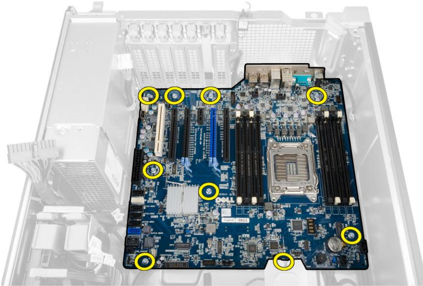
5. Lift the system board in an upward direction and remove it from the computer.
