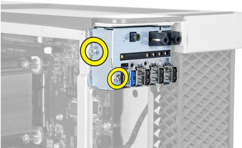
4. Remove the USB 3.0 module from the chassis.
