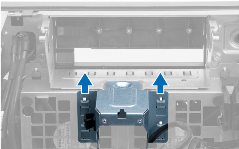
6. Lift the metal plate out of the chassis.
