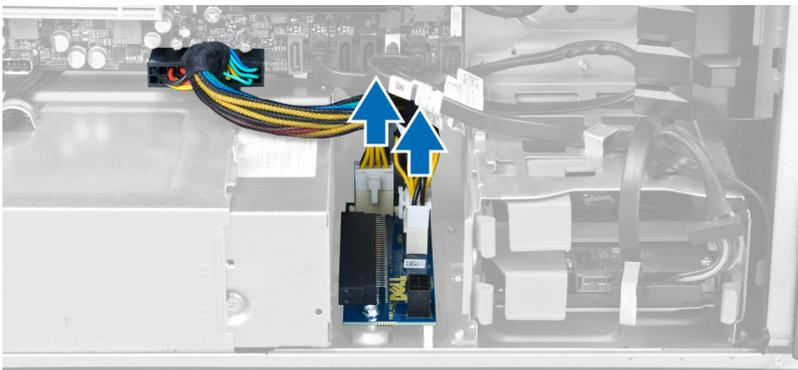
6. Remove the screws securing the PSU card to the slot.
