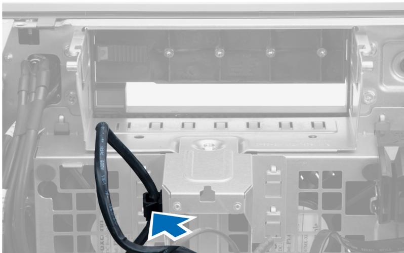
4. Remove the screw that secures metal plate to the system fan.
