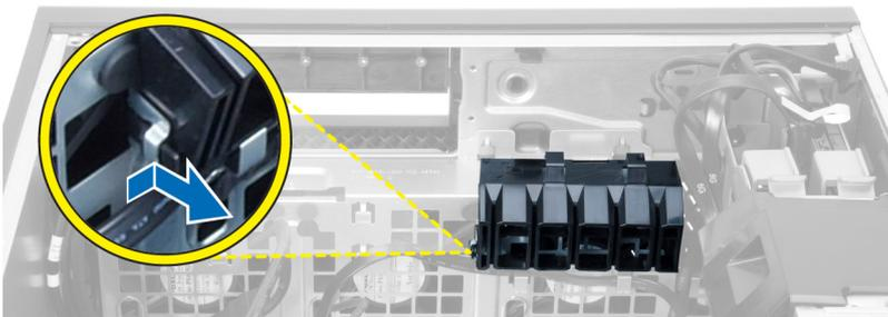
9. Remove the air baffle out of the computer.
