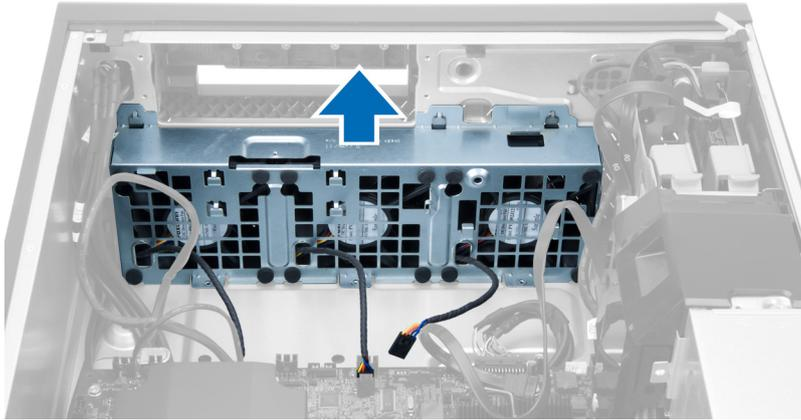
13. Pry away the grommets to remove the system fans from the system-fan assembly.
