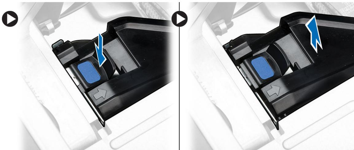
4. Repeat **Step 3** to remove the second air tunnel module from the computer.
