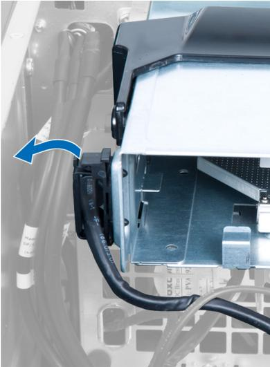
6. Press down on the latch and lift up the cables.
