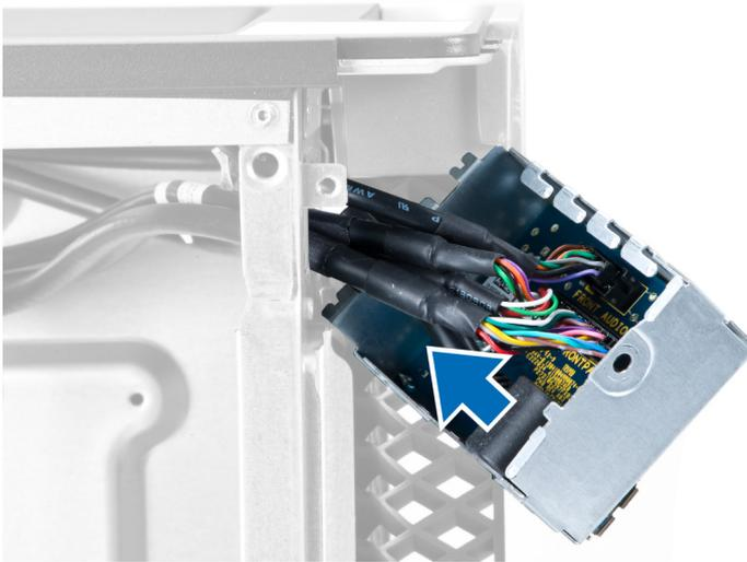
5. Disconnect the cables to release the I/O panel.
