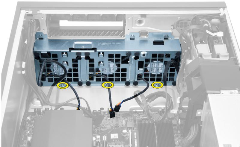
12. Lift the system-fan assembly from the chassis.
