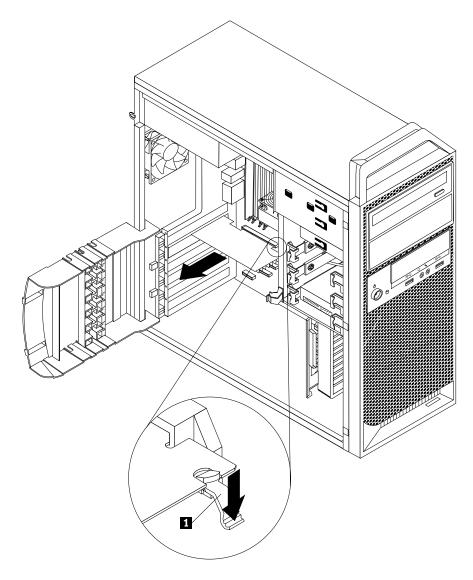
Figure 9. Removing a PCI card
