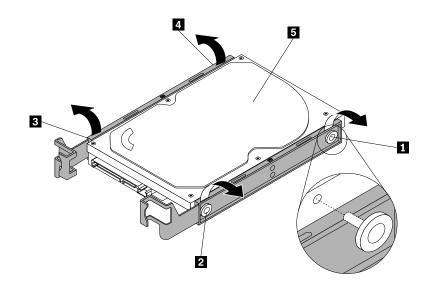
Figure 29. Installing the hard disk drive into the bracket
