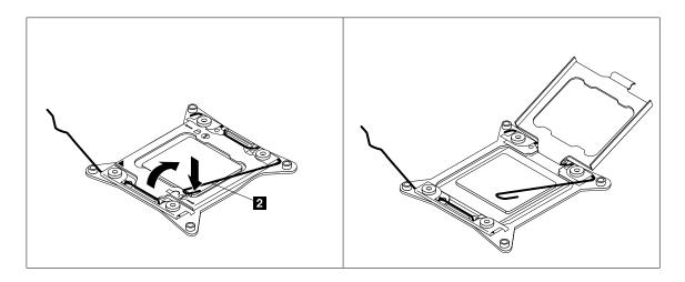
Figure 39. Opening the microprocessor retainer
