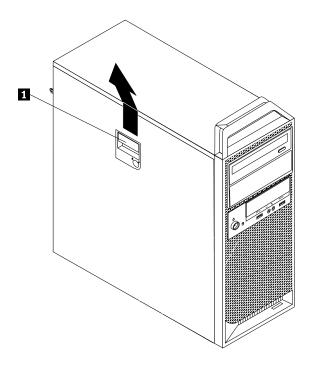
Figure 6. Removing the computer cover
