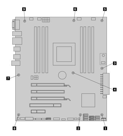
Figure 45. Removing the nine screws that secure the system board to the chassis
