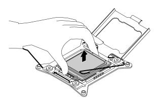
Figure 40. Removing the microprocessor
