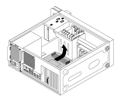
Figure 46. Removing the system board
