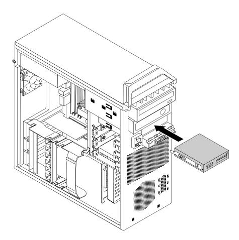
Figure 22. Installing the card reader
