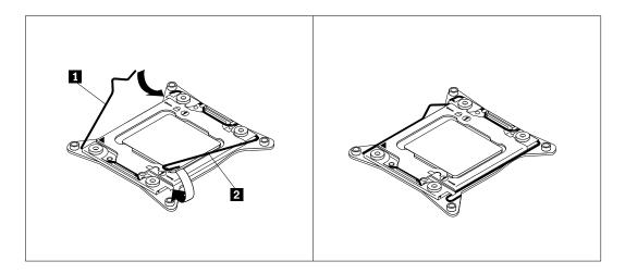
Figure 44. Securing the microprocessor in the socket
