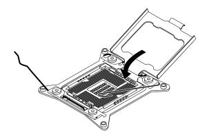
Figure 47. Closing the microprocessor retainer
