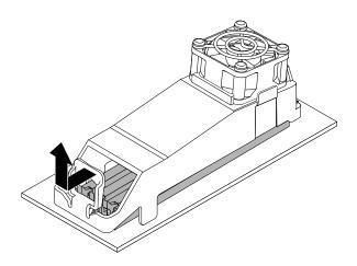
Figure 11. Removing the memory cooler
