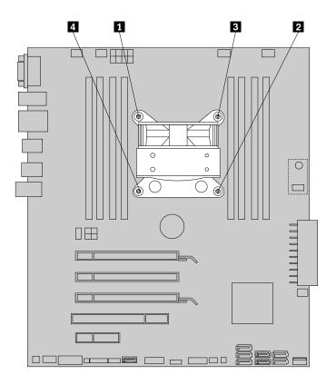
Figure 25. Removing the heat sink and fan assembly
