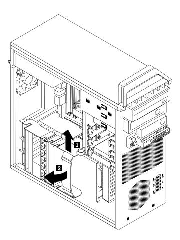
Figure 8. Opening the adapter card retainer
