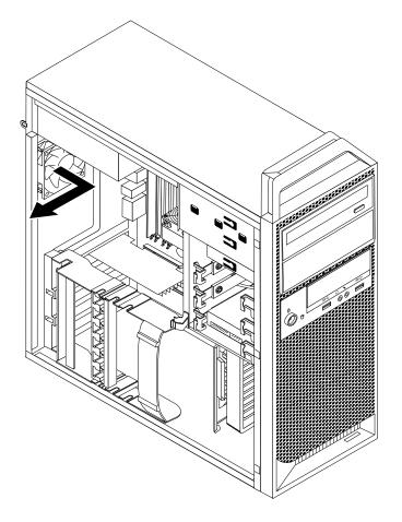
Figure 26. Removing the rear fan assembly
