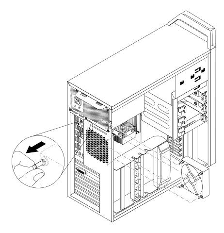
Figure 27. Installing the rear fan assembly
