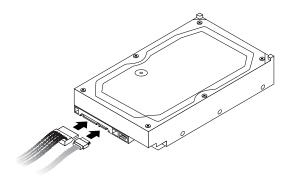
Figure 32. Connecting a SATA hard disk drive
