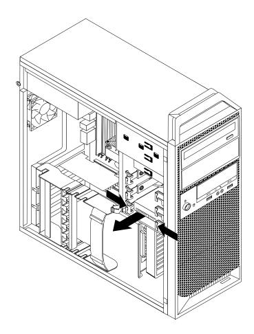
Figure 28. Removing a hard disk drive
