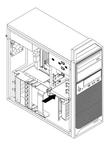
Figure 31. Installing a hard disk drive
