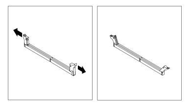
Figure 13. Opening the retaining clips
