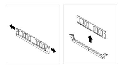
Figure 12. Removing a memory module
