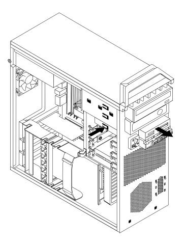
Figure 20. Removing the card reader
