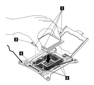
Figure 42. Installing the microprocessor
