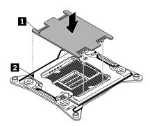
Figure 49. Installing the microprocessor socket cover
