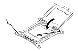
Figure 43. Closing the microprocessor retainer
