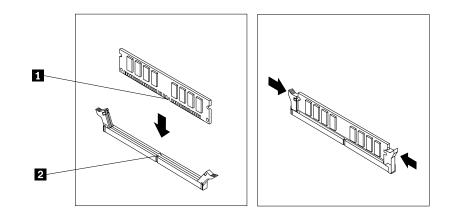
Figure 14. Installing a memory module
