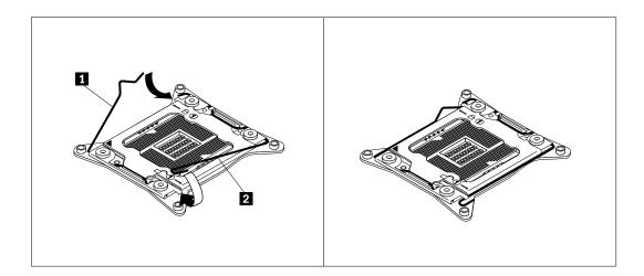
Figure 48. Securing the microprocessor in the socket
