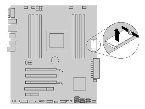
Figure 34. Removing the hard disk drive enablement module
