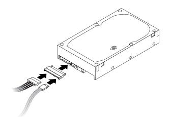
Figure 33. Connecting a SAS hard disk drive
