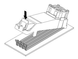
Figure 15. Installing the memory cooler
